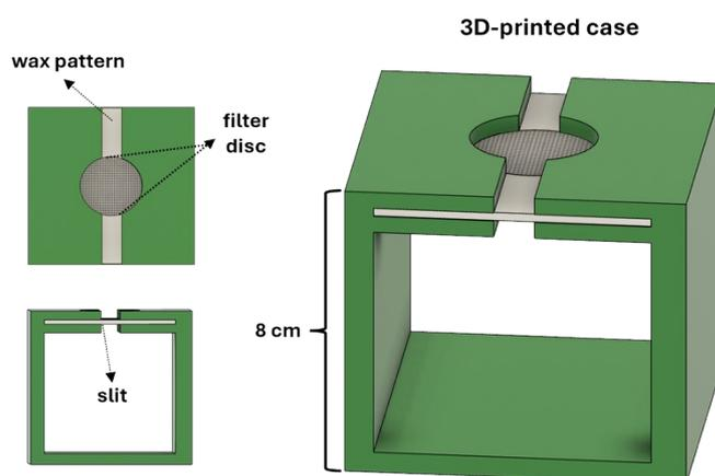
**Figure S1:** The 3D-printed case served as the platform for the reaction on the paper-based platform. The device included a slit to facilitate the handling of the filter disc. The paper platform consisted of a wax pattern, i.e. hydrophobic area, for liquid control and the deposition of the reagents and a circle pattern, i.e. hydrophilic area, where the reaction was performed.
