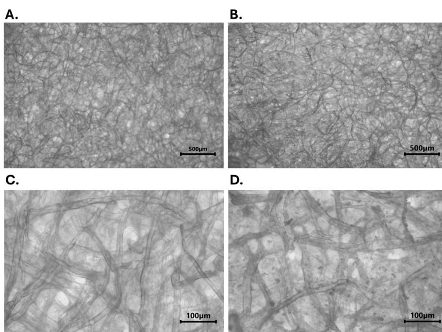
**Figure S3:** Microscope images of the paper-based platform before (A, C) and after the reaction and product removal (B, D) at two different scales: 500  $\mu\text{m}$  and 100  $\mu\text{m}$ .
