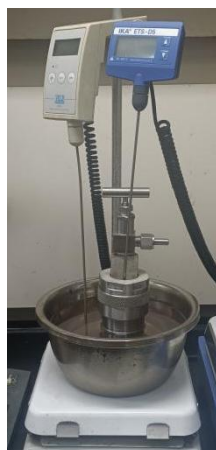
Figure S1. Hydrothermal reactor with temperature sensor.
