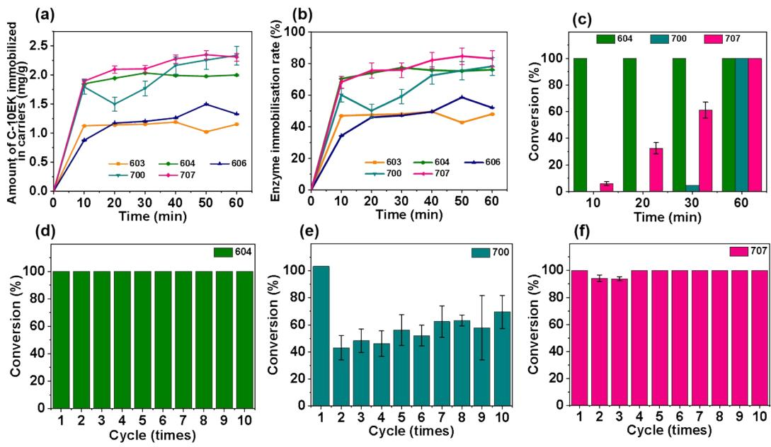
**Fig. S5** Lysine decarboxylase immobilization amount (a) and immobilization rate (b) of five kinds of resins Catalytic efficiency (c) and cyclic stability (d, e, f) of the three immobilized enzymes
