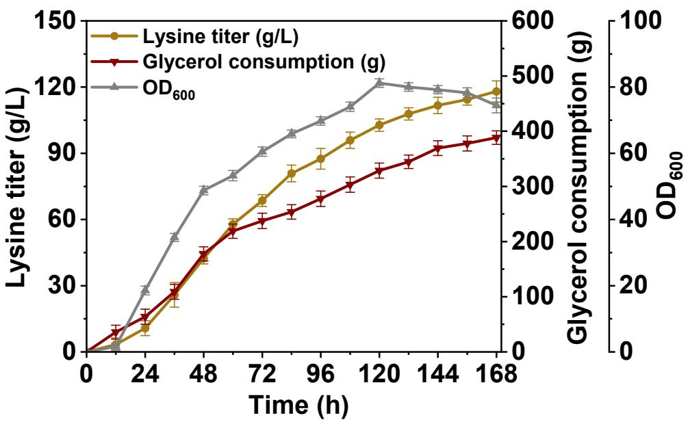
**Fig. S8** Fed-batch fermentation profiles cgl-FDK-VIII in a 5 L bioreactor. Time profiles of OD<sub>600</sub>, glycerol consumption, lysine yield were shown during the fed-batch cultivation. Values were shown as mean  $\pm$  SD ( $n = 3$ )
