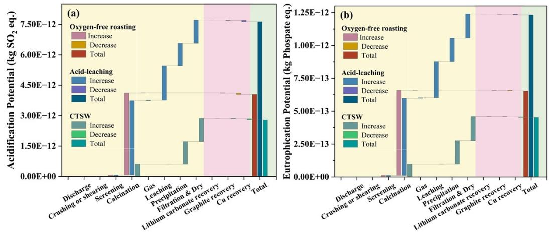
**Fig. S5** Comparison of environmental impact between CTS, acid leaching, and conventional roasting process for utilizing spent graphite based on life cycle assessment
