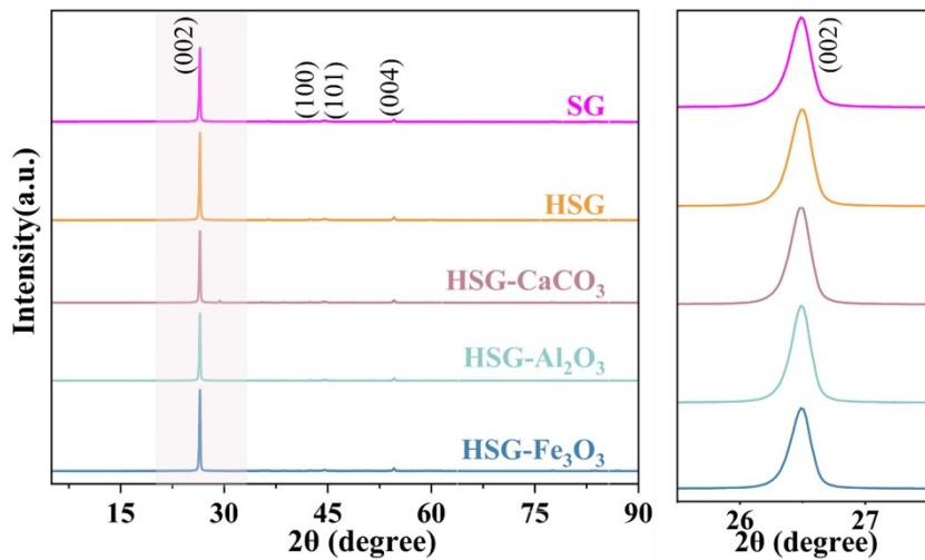
**Fig. S2** XRD patterns of spent graphite, HSG without medium, and HSG samples with different mediums.
