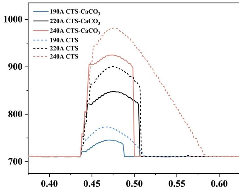
**Fig. S1** Time-temperature relationship of heating procedure in direct CTS and with added  $\text{CaCO}_3$  medium conditions (fast mode, time parameter set to 5s).
