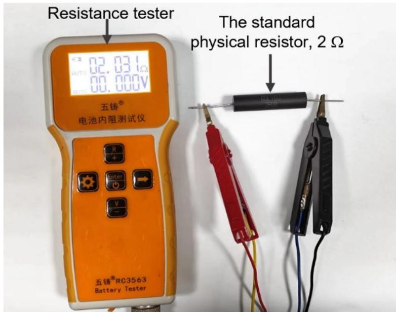
**Fig. S12.** A standard physical resistor (2.031  $\Omega$  measured by a four-electrode resistance tester, RC3563, Wuzhu, China).
