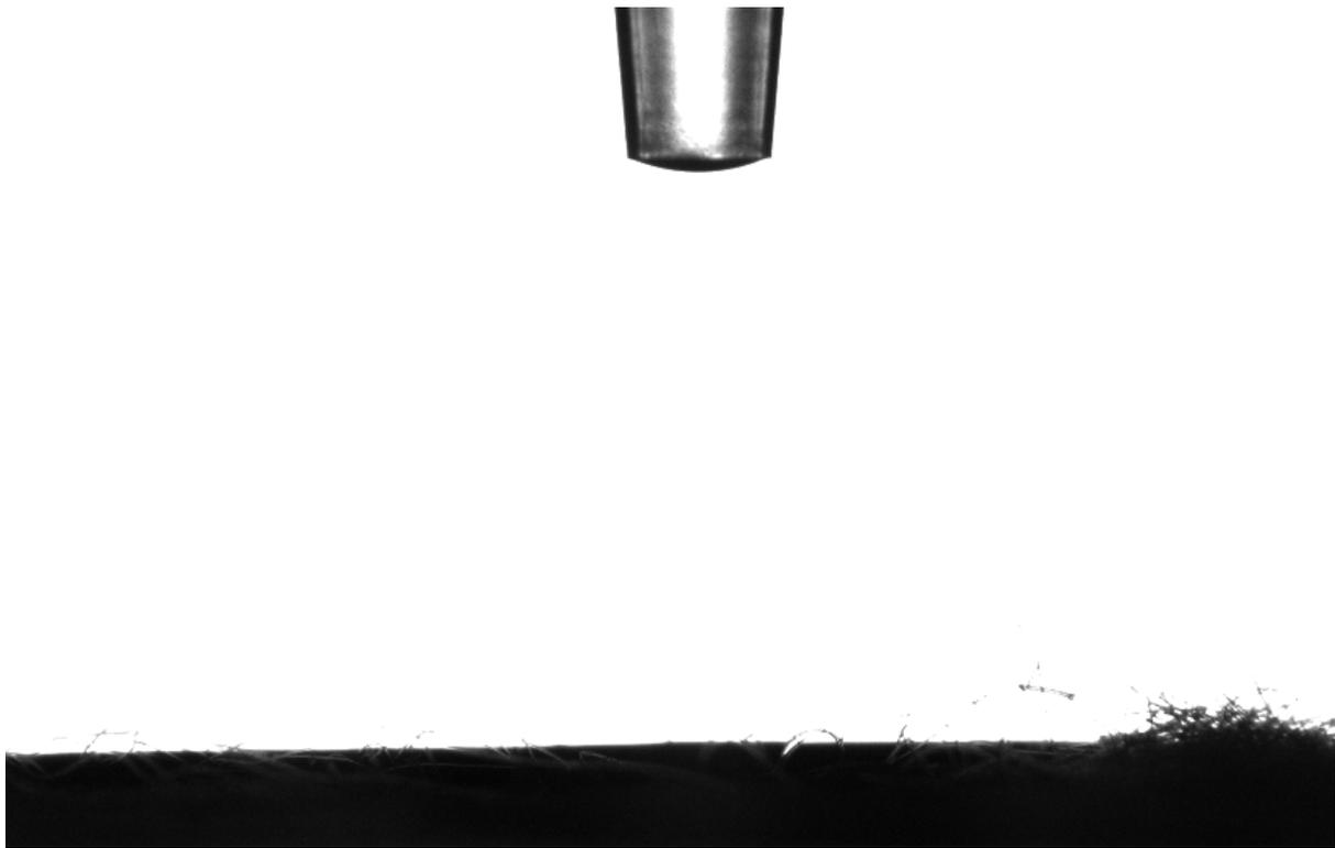
**Figure S7.** Water contact angle measurement of plain cellulose as soon as exposing to the water droplet.
