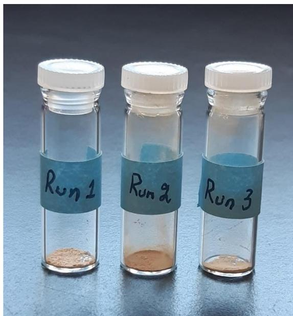
**Fig. S33 SGHT-200 after multiple runs in the reductive cleavage of 2-(2-methoxyphenoxy)-1-phenylethanone (PPEn) under blue light (440 nm).**
