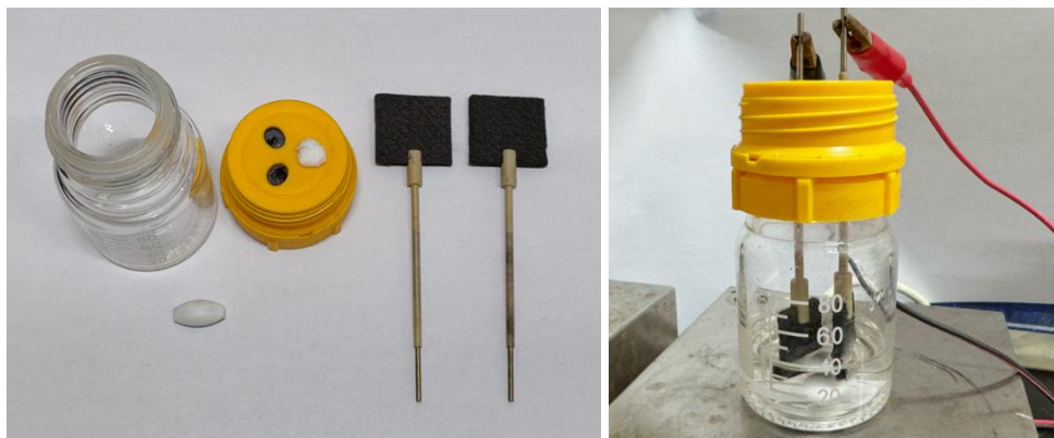
Figure S2. Electrolysis setup for the gram scale experiment.
