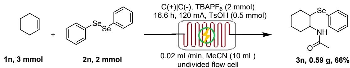
In air, **1n** (304 µL, 3 mmol), **2n** (0.625 g, 2 mmol), TBAPF<sub>6</sub> (0.775 g, 2 mmol), TsOH (86.1 mg, 0.5 mmol), and MeCN (10 mL) were mixed and then aspirated into a syringe. A flow electrochemical reactor, equipped with graphite plates as both the anode and cathode, was used, with the surface area of the graphite plates measuring 8 cm×6 cm. The mixture underwent flow
