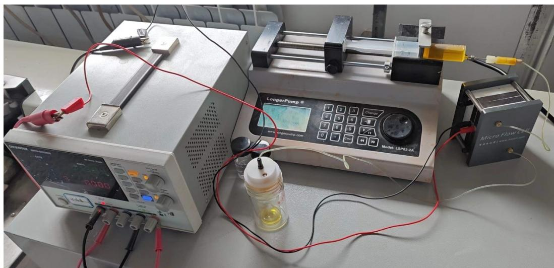
**Fig. S3** Flow electrochemical reactor for scale-up experiment
