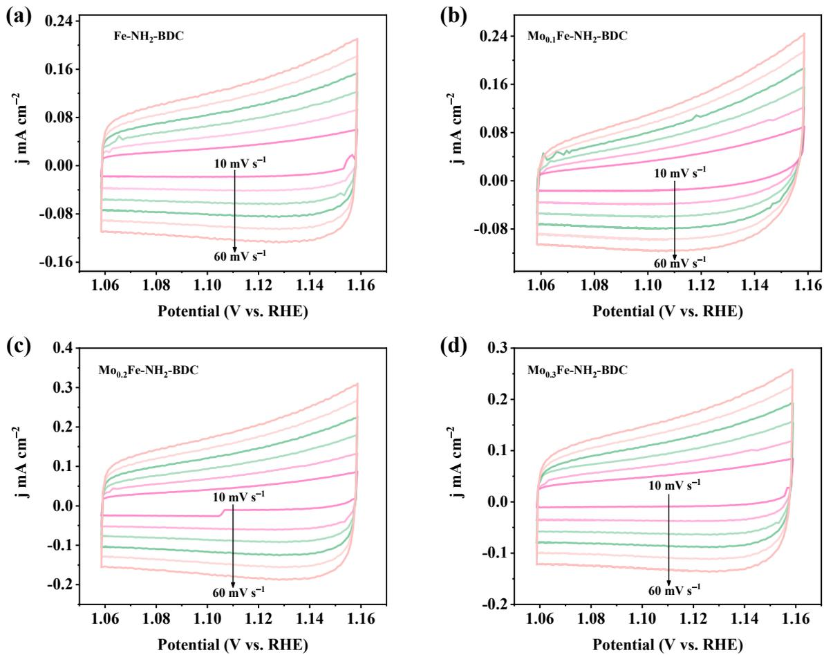
**Fig. S4.** CV curves of (a) Fe-NH<sub>2</sub>-BDC, (b) Mo<sub>0.1</sub>Fe-NH<sub>2</sub>-BDC, (c) Mo<sub>0.2</sub>Fe-NH<sub>2</sub>-BDC, and (d) Mo<sub>0.3</sub>Fe-NH<sub>2</sub>-BDC operated in non-Faradaic potential window with different scan rates (10-60  $\text{mV s}^{-1}$ ).
