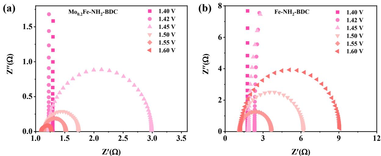
**Fig. S6.** Nyquist plots for (a) Mo<sub>0.2</sub>Fe-NH<sub>2</sub>-BDC and (b) Fe-NH<sub>2</sub>-BDC at different applied potentials.
