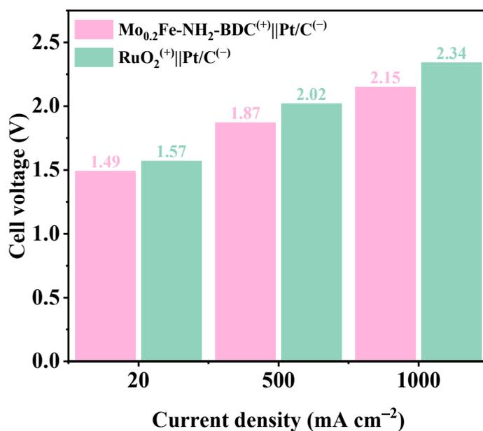
**Fig. S9.** Comparison of cell voltages required at varying current densities for  $\text{Mo}_{0.2}\text{Fe-NH}_2\text{-BDC}^{(+)} \parallel \text{Pt/C}^{(-)}$  and  $\text{RuO}_2^{(+)} \parallel \text{Pt/C}^{(-)}$  systems.
