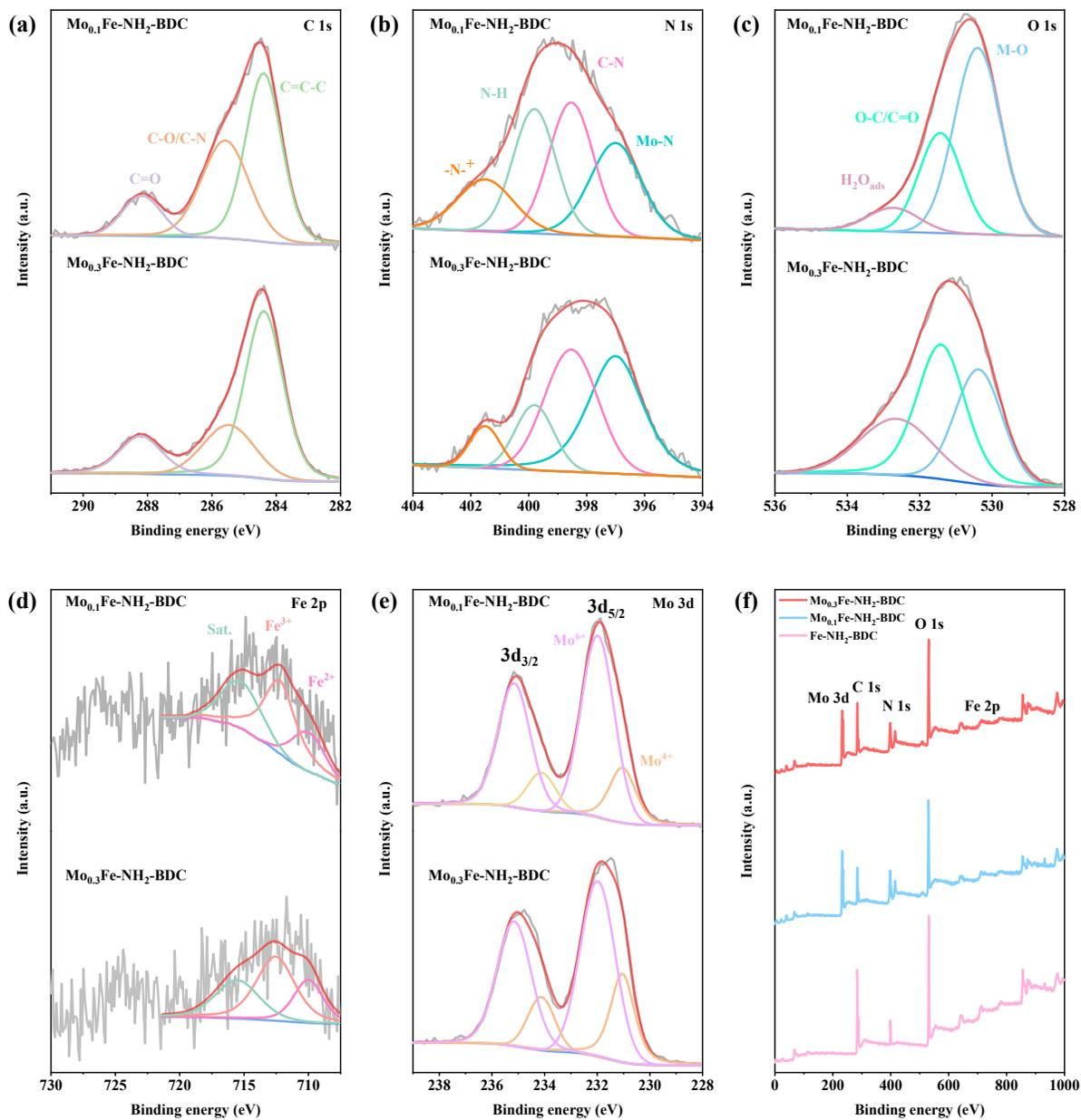
**Fig. S3.** High-resolution XPS spectra of (a) C 1s, (b) N 1s, (c) O 1s, (d) Fe 2p, (e) Mo 3d, and (f) XPS survey for  $\text{Fe-NH}_2\text{-BDC}$ ,  $\text{Mo}_{0.1}\text{Fe-NH}_2\text{-BDC}$  and  $\text{Mo}_{0.3}\text{Fe-NH}_2\text{-BDC}$ .
