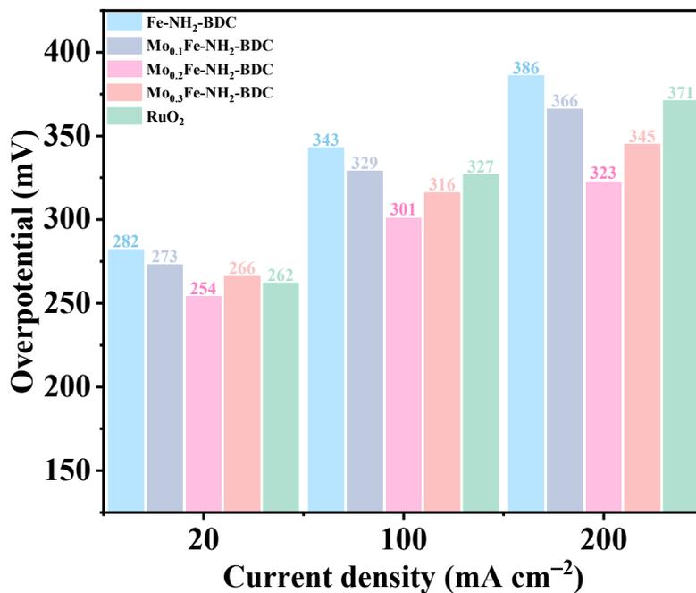
**Fig. S5.** Overpotential comparison of Fe-NH<sub>2</sub>-BDC, Mo<sub>x</sub>Fe-NH<sub>2</sub>-BDC (x = 0.1, 0.2, 0.3), and RuO<sub>2</sub> at 20, 100, and 200 mA cm<sup>-2</sup>.
