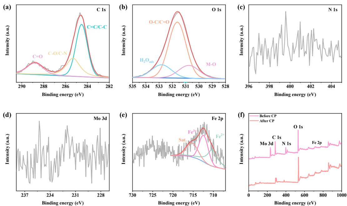
**Fig. S8.** High-resolution XPS spectra of (a) C 1s, (b) N 1s, (c) O 1s, (d) Fe 2p, (e) Mo 3d, and (f) XPS survey of  $\text{Mo}_{0.2}\text{Fe-NH}_2\text{-BDC}$  after stability test.
