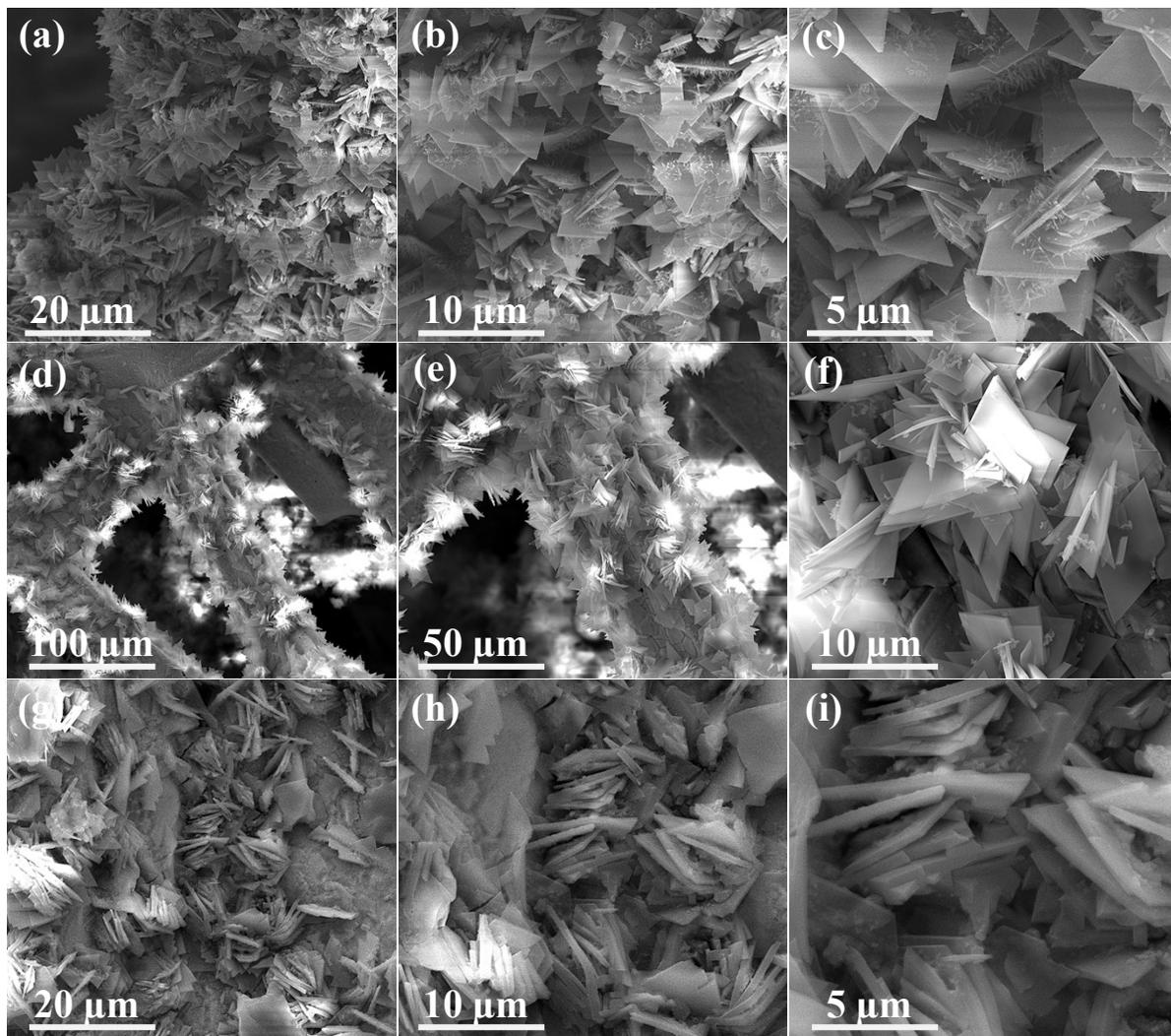
**Fig. S1.** SEM images of (a-c) Mo<sub>0.1</sub>Fe-NH<sub>2</sub>-BDC, (d-f) Mo<sub>0.2</sub>Fe-NH<sub>2</sub>-BDC, and (g-i) Mo<sub>0.3</sub>Fe-NH<sub>2</sub>-BDC
