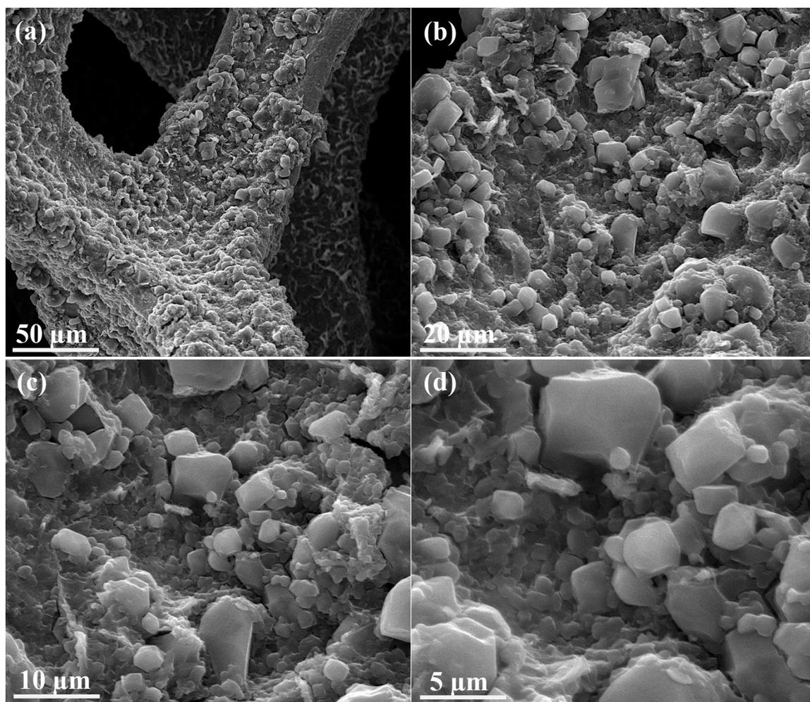
**Fig. S7.** SEM images of (a-d)  $\text{Mo}_{0.2}\text{Fe-NH}_2\text{-BDC}$  after OER stability test.
