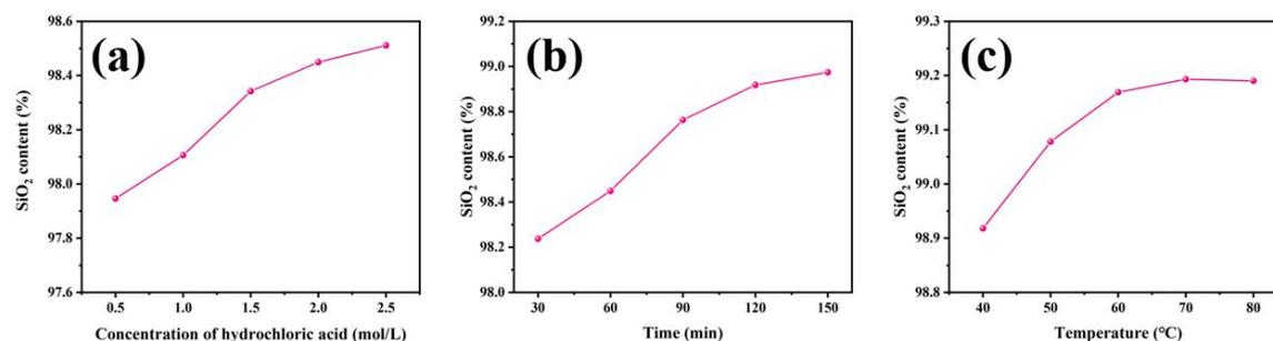
Fig.1(a) Effect of acid concentration on SiO<sub>2</sub> content, (b) Effect of reaction time on SiO<sub>2</sub> content,
