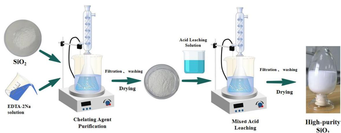
Fig. 4. Schematic diagram of impurity removal by chelating agents and mixed acid leaching for the preparation of high-purity SiO<sub>2</sub>
