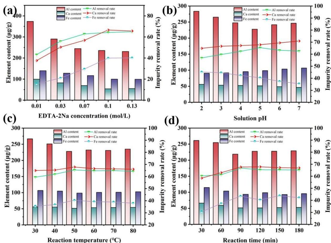
**Fig. 5.** Effects of process parameters on impurity content and removal rate of SiO<sub>2</sub>: (a) EDTA-2Na concentration, (b) Solution pH, (c) Reaction temperature, (d) Reaction time
