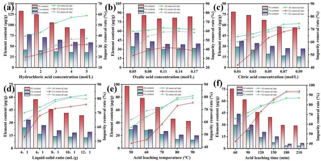
Figure 5 Effects of acid leaching conditions on impurity content and removal rate of SiO<sub>2</sub>: (a) hydrochloric acid concentration, (b) oxalic acid concentration, (c) citric acid concentration, (d) liquid-to-solid ratio, (e) acid leaching temperature, (f) acid leaching time
