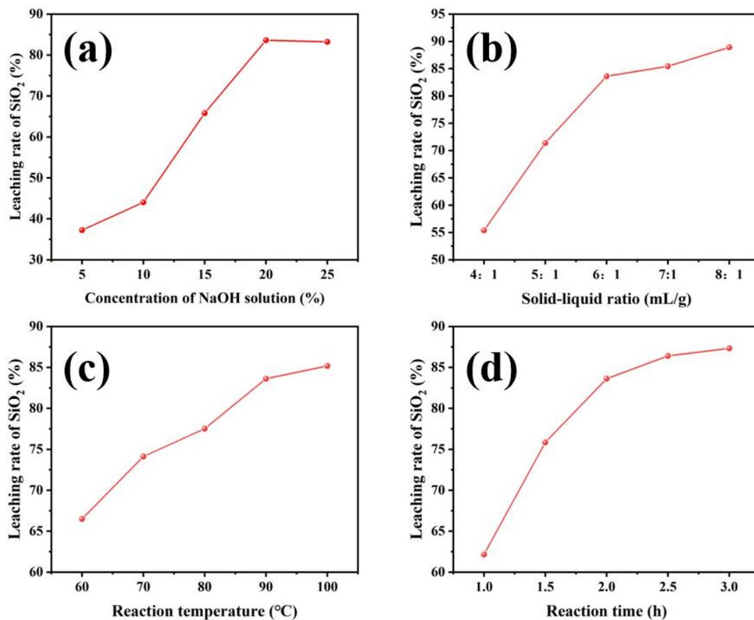
Fig.2 (a) Effect of sodium hydroxide mass fraction on the leaching rate of SiO<sub>2</sub>, (b) Effect of reaction time on the leaching rate of SiO<sub>2</sub>, (c) Effect of reaction temperature on the leaching rate of SiO<sub>2</sub>, (d) Effect of reaction time on the leaching rate of SiO<sub>2</sub>
