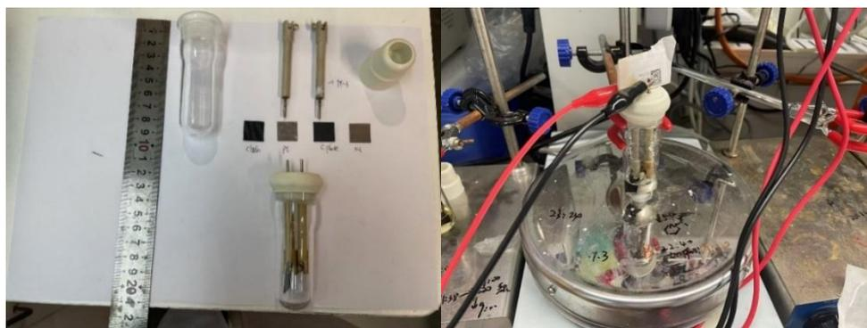
**Figure S3** Batch electrolysis setups.
