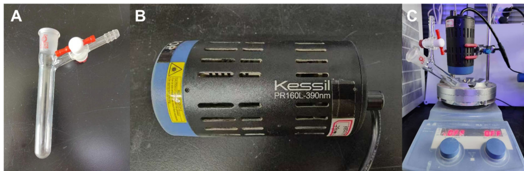
Figure S1. Photographs of the reaction vessel, Kessil lamp, and photoreaction device. A: 25 mL reaction vial; B: Kessil PR160L-390 nm lamp, C: photoreactor.
