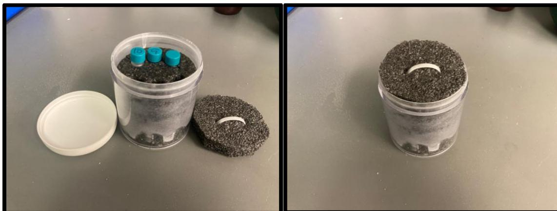
**Figure S3:** Custom formed closed cell polyethylene foam holder, allowing for simultaneous screening of six reactions. Enclosed vessel and tight fit of vessels is important to stabilize vials. Setup was used exclusively for screening conditions. Due to the possibility of vial movement, all experiments were validated and reported in PTFE bottles.
