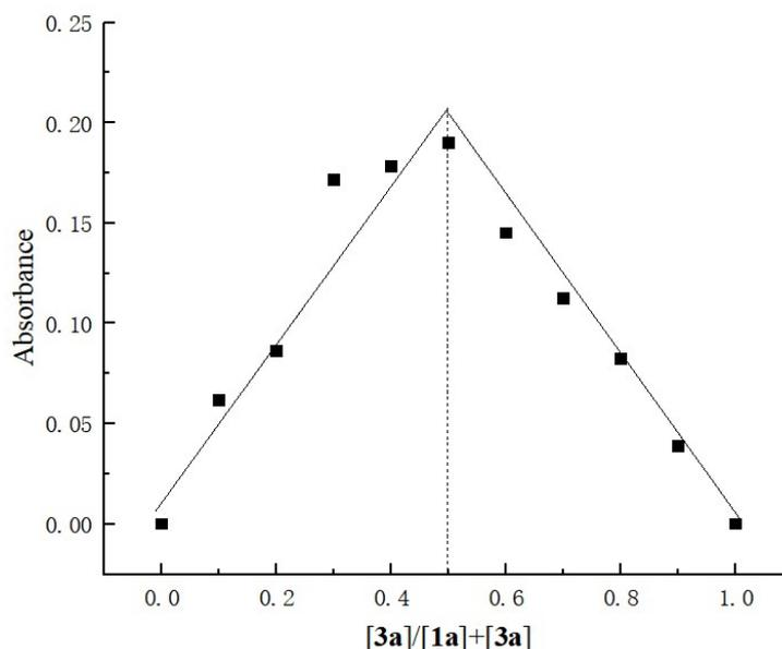
Figure S4. Job's plot between PhSO<sub>2</sub>Ph (**1a**) and C<sub>4</sub>F<sub>9</sub>I (**3a**).
