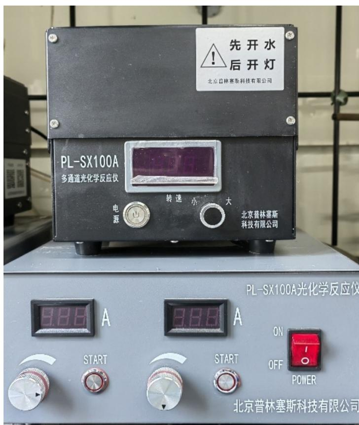
**Figure S1.** Photograph of the photoreactor used for the reaction (distance from light source to the reaction tube: 2.0 cm; power: 10 W).
