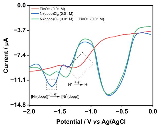
**Figure S4:** The SWV curve of  $\text{Ni}(\text{dppp})\text{Cl}_2$ , PivOH and  $\text{Ni}(\text{dppp})\text{Cl}_2$  with PivOH
