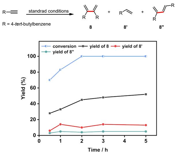
**Figure 12.** Kinetic study. The yields of products were determined by <sup>1</sup>H-NMR analysis using 1,3,5-trimethoxybenzene as the internal standard.
