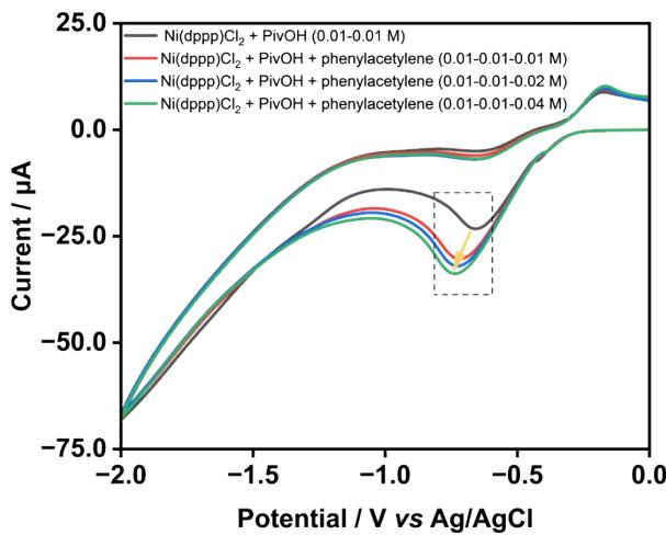
**Figure S2:** The effect of adding PivOH and phenylacetylene on the CV curve of  $\text{Ni}(\text{dppp})\text{Cl}_2$
