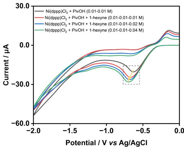
**Figure S3:** The effect of adding PivOH and 1-hexyne on the CV curve of  $\text{Ni}(\text{dppp})\text{Cl}_2$
