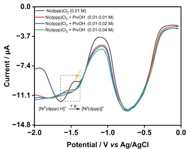
**Figure S5:** Effect of adding different concentrations of PivOH on SWV curve of  $\text{Ni}(\text{dppp})\text{Cl}_2$
