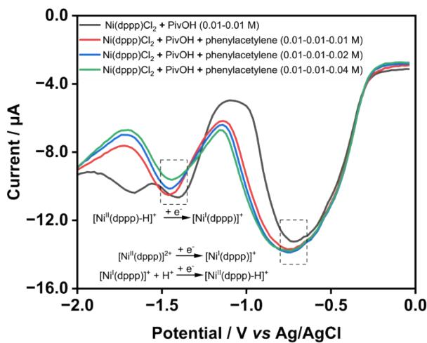
**Figure S6:** The effect of adding PivOH and phenylacetylene on the SWV curve of  $\text{Ni}(\text{dppp})\text{Cl}_2$
