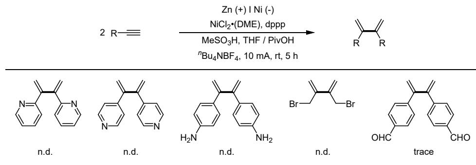
**Scheme S1:** Standard reaction conditions: zinc plate (1.5 cm × 1.5 cm × 0.03 cm) as the anode and the nickel plate (1.5 cm × 1.5 cm × 0.05 cm) as the cathode, constant current = 10 mA, **1** (0.3 mmol), NiCl<sub>2</sub>·(DME) (20 mol%), 1,3-bis(diphenylphosphaneyl)propane(dppp) (24 mol%), <sup>7</sup>Bu<sub>4</sub>NBF<sub>4</sub> (0.6 mmol), THF (6.0 mL), MeSO<sub>3</sub>H (1.5 equiv.), PivOH (10.0 equiv.), undivided cell, N<sub>2</sub>, 28 °C, 5 h.
