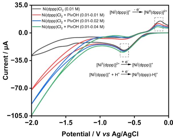
**Figure S1:** Effect of adding different concentrations of PivOH on CV curve of  $\text{Ni}(\text{dppp})\text{Cl}_2$
