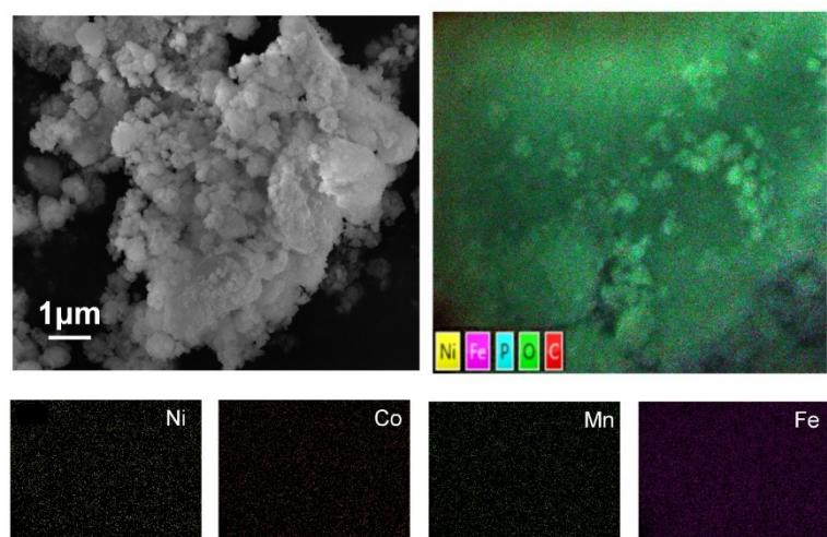
**Figure S15** SEM-EDS images of leaching residues after roasting at 600°C for 20 min.
