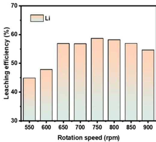
**Figure S6** Effect of milling rotation speed on the water leaching efficiency of milling products. (Factorial experiments, other than the exploratory factor, were conditioned on solid-liquid ratio: 5 g/L, temperature: 90 °C, time: 60 min, ball powder ratio: 50: 1, rotation speed: 750 rpm, milling time: 7 h).
