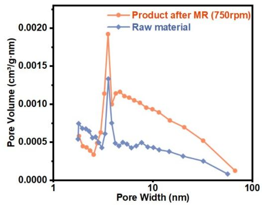
**Figure S2** Pore width distribution of samples before and after MR.
