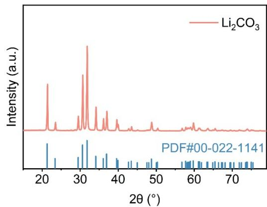
**Figure S12** XRD pattern of recovered  $\text{Li}_2\text{CO}_3$ .
