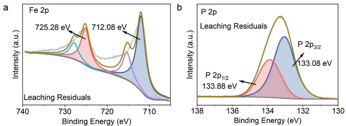
**Figure S16** XPS spectra of (a) Fe2p and (b) P 2p of leaching residues after roasting at 600°C for 20 min.
