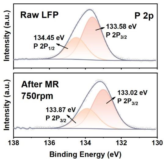
**Figure S3** XPS spectra of P 2p in products without and after MR.
