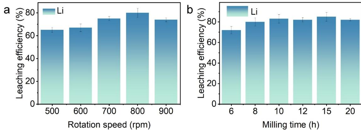
**Figure S5** Effect of (a) rotation speed and (b) milling time on the water leaching efficiency of milling product.
