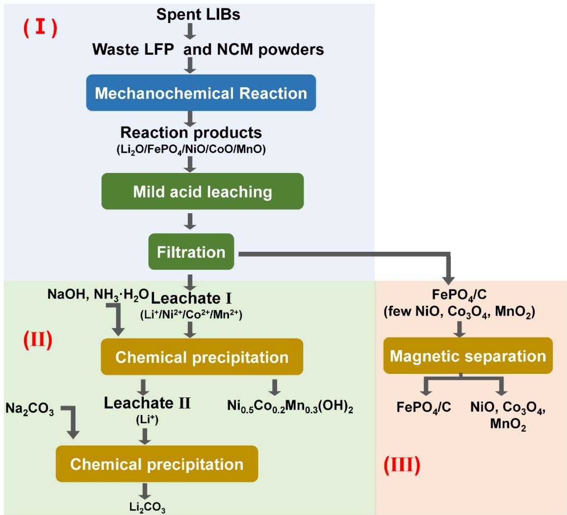
**Figure S1** The flow chart of proposed green route for recovery of valuable metals from spent LIBs.
