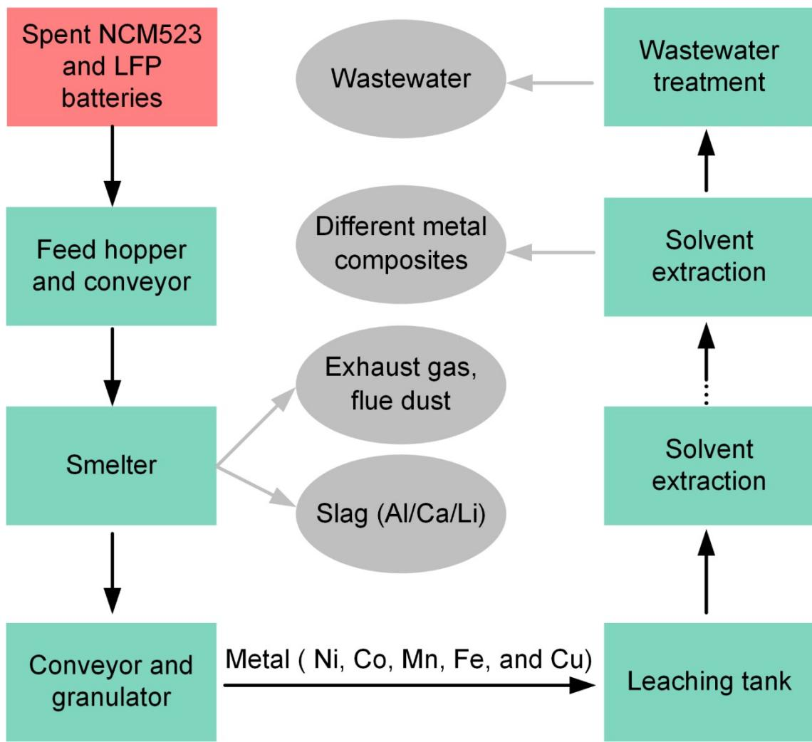
**Figure S19** Schematic of Pyro recycling.
