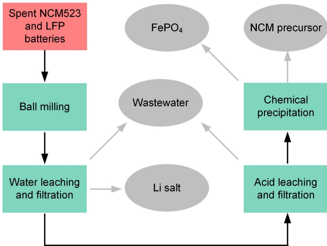
**Figure S21** Schematic of this work.
