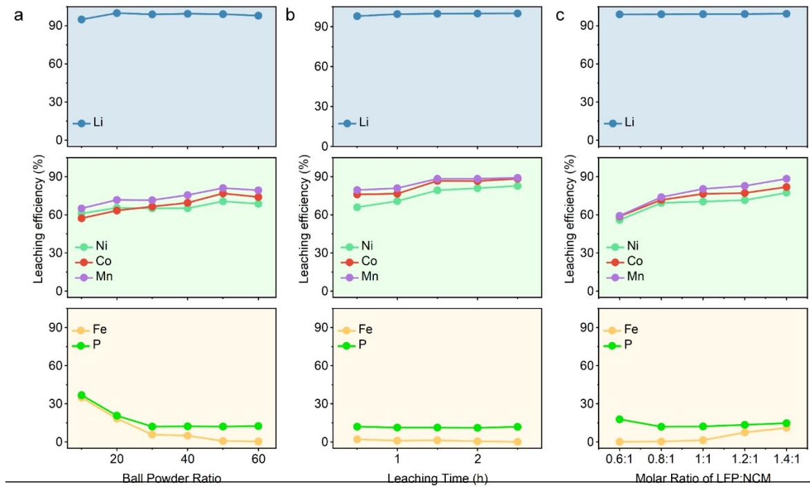
**Figure S8** Effect of (a) ball powder ratio, (b) leaching time, and (c) molar ratio of LFP: NCM on leaching efficiency.
