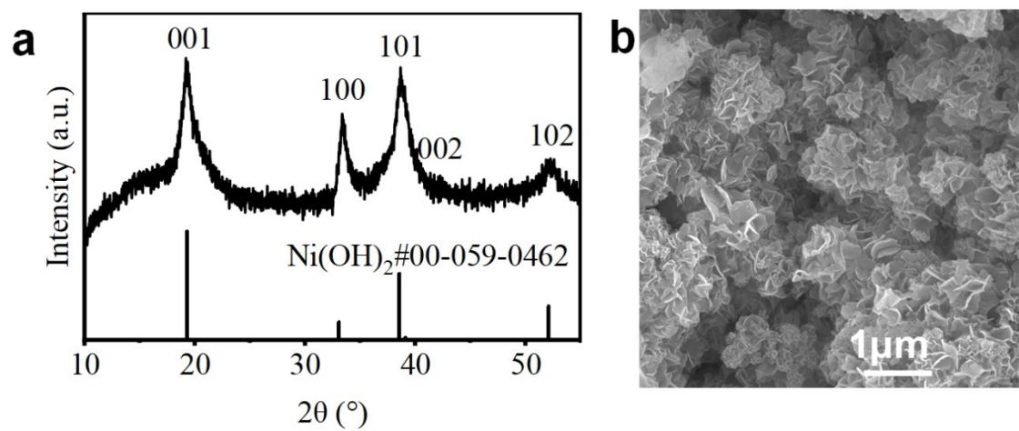
**Figure S18** (a) XRD pattern and (b) SEM image of the  $\text{Ni}_{0.5}\text{Co}_{0.2}\text{Mn}_{0.3}(\text{OH})_2$ .
