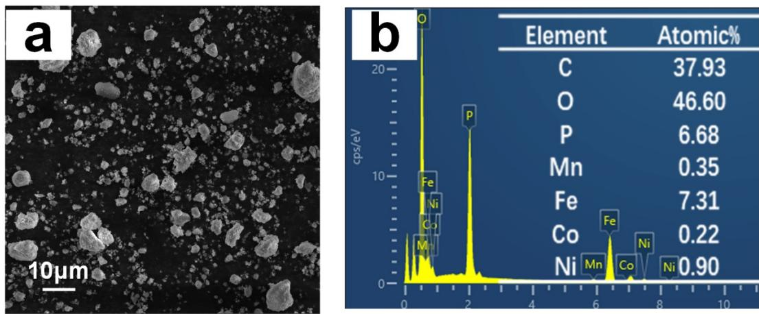
**Figure S14** SEM-EDS images of leaching residues after roasting at 600°C for 20 min.
