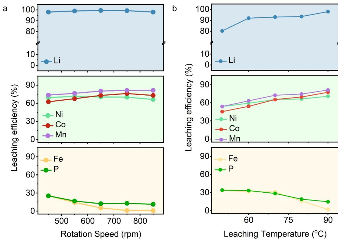
**Figure S9** Effect of (a) rotation speed, and (b) temperature on leaching efficiency.
