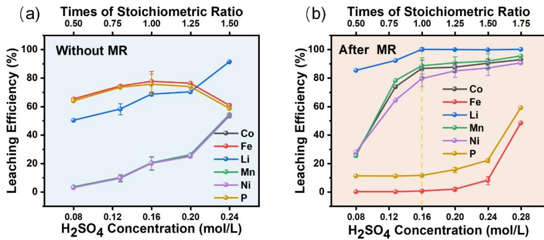
**Figure S7** Leaching efficiency of samples at different acid concentrations (a) without and (b) after MR.
