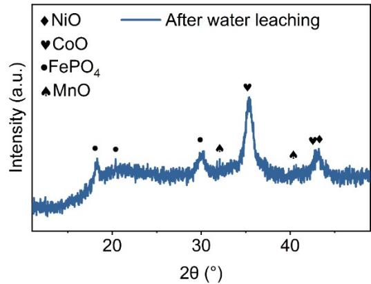
**Figure S13** XRD pattern water leaching residues.
