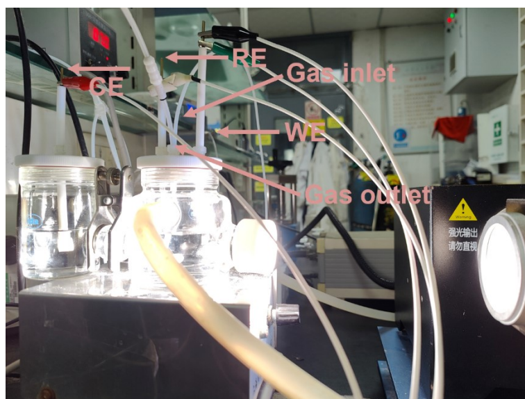
Fig. S3 H-type electrolytic cell used for photoelectrocatalytic CO 2 reduction.
