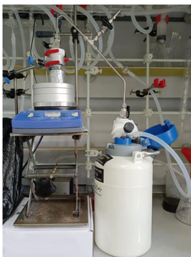
Figure S5. The reaction device for the depolymerization via intermittent evaporation
