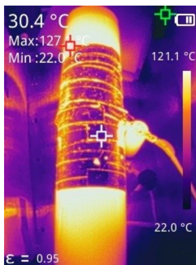
Figure S2. Maximum reaction temperature measured by an infrared thermal camera.
