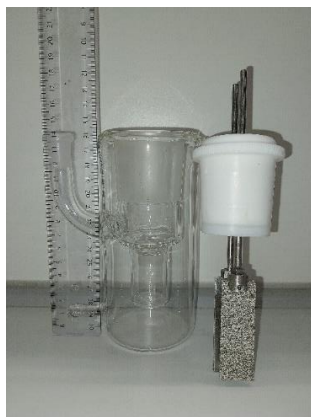
Figure S1 Undivided glass cells with a volume of 25 mL equipped with a cooling jacket available as SynLectro™ 25mL (Merck S.A, an affiliate of Merck KGaA, Darmstadt, Germany), two electrodes (interelectrode gap: 12 mm) and a cross-shaped stirring bar. 1 Cathode material consists of a stainless-steel VA1.4571 electrode and a nickel foam RCM-Ni4753.03 anode (Recemat™, Dodewaard, Netherlands).
