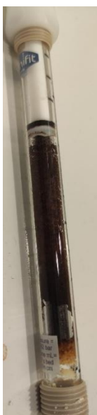
Fig. SI. 4. a) ^1\text{H} -NMR follow-up of the dehydration of fructose into HMF using \text{CHCl}_3 as internal standard by in-line NMR using Magritek Spinsolve 80 Ultra. b) appearance of the catalyst after performance of the flow reaction c) stability of the catalyst to produce HMF using fructose (10 wt%) T = 120^\circ\text{C} , 50\ \mu\text{L}/\text{min} of water solution, 200\ \mu\text{L}/\text{min} 2-MeTHF using a HPLC piston pumps
