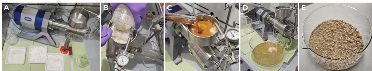
Figure S2. Photographs taken during 1.0 mol scale amidation of 4-hydroxyphenylacetic acid with 3,5-dimethylaniline. (A) Reagents weighed and prepared. (B) Feeding the carboxylic acid/EDC·HCl/EtOAc mixture. (C) Adding the aniline component. (D) Collection of crude material. (E) Isolated amide product 3 .
