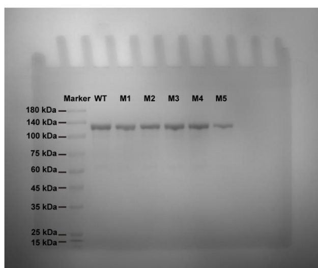
Fig. S4 SDS-PAGE of CYP102A1 and its mutants. Lane 1 is the marker and lane 2 to 7 are purified enzymes WT, M1, M2, M3, M4 and M5 respectively.
