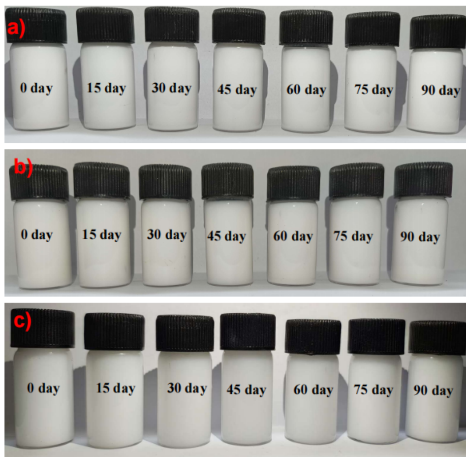
Figure S2 Colour photographs of [Cho][Ole] ILs emulsion a) containing EMIm EtSO 4 , b) emulsion containing [P 66614 ][Dec] and c) CTAB containing EMIm EtSO 4 for 90 days.
