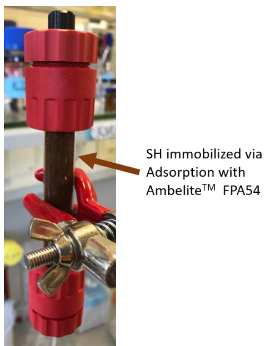
Fig. S19. NADH regeneration unit consisting of a column packed with amberlite resin, on which soluble hydrogenase (SH) and catalase were immobilized for cofactor regeneration.
