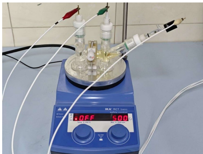
Fig. S11. Reaction setup for electrochemical semi-hydrogenation of alkynes.
