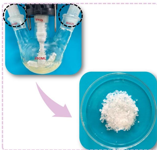
Figure S18. White sublimate formed during the polyesterification process.
