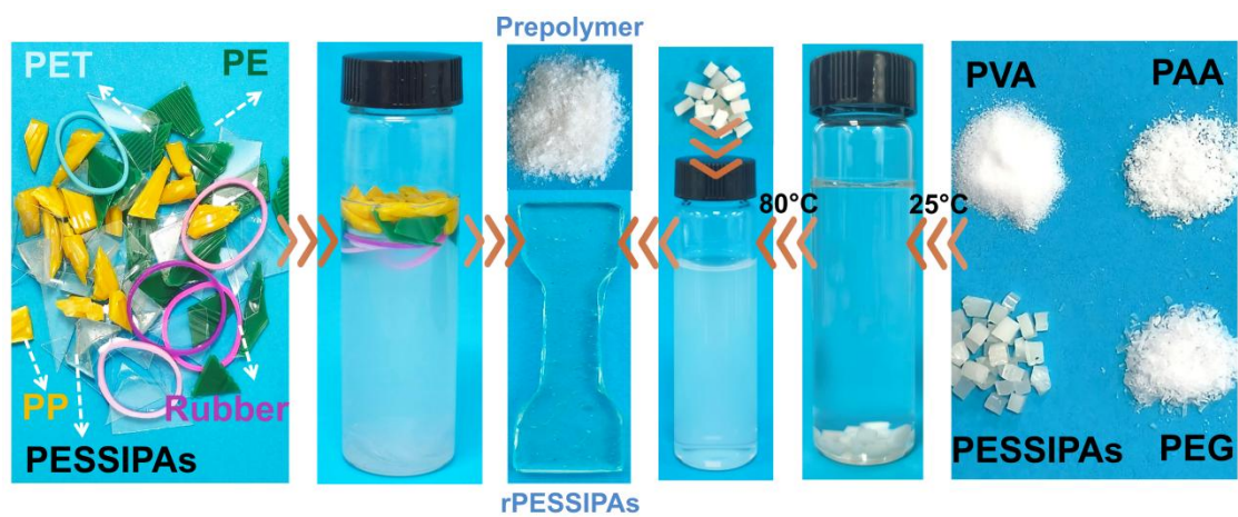
Figure S45. Approach to recycle PESSIPA0.1 from mixed plastics. Solvent: water.
