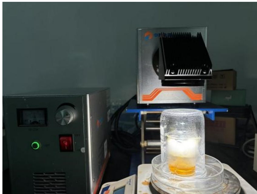
Fig. S1 The schematic diagram of solar driven evaporation device.
