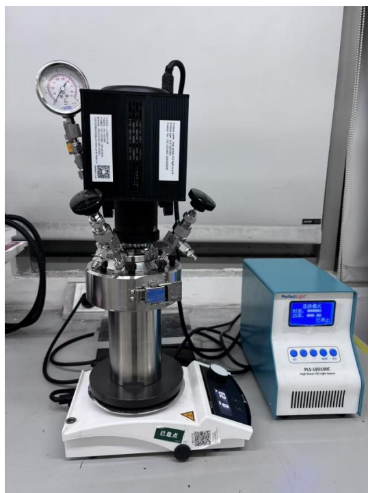
Figure S4. Image of the laboratory-scale high-pressure batch photoreactor used for methane functionalization experiments.
