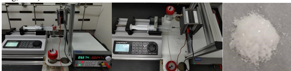
Figure S6. Electrochemical reaction equipment for 5a in continuous flow reactor
