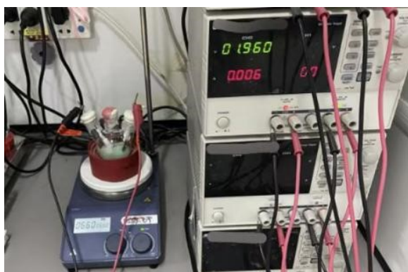
Figure S2. Electrochemical gram-scale reaction equipment for 3a in batch reactor
