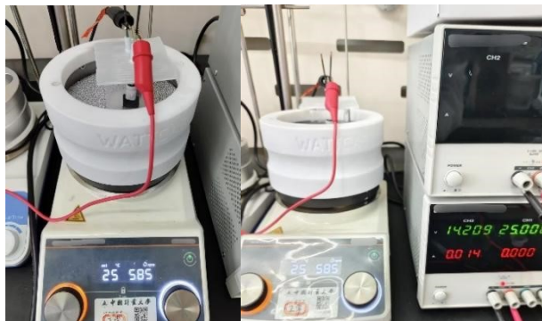
Figure S3. Electrochemical gram-scale reaction equipment for 5a in batch reactor
