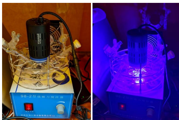
Figure S1. Photograph of the photocatalytic reactor
