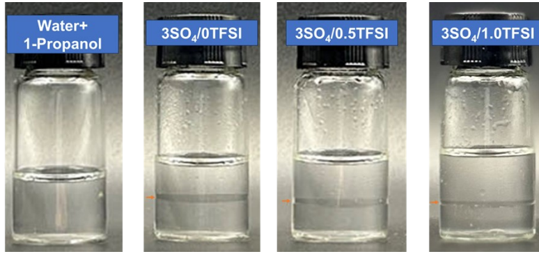
Fig. S4 Digital photos of biphasic liquid electrolytes with various \text{Zn}(\text{TFSI})_2 concentrations.
