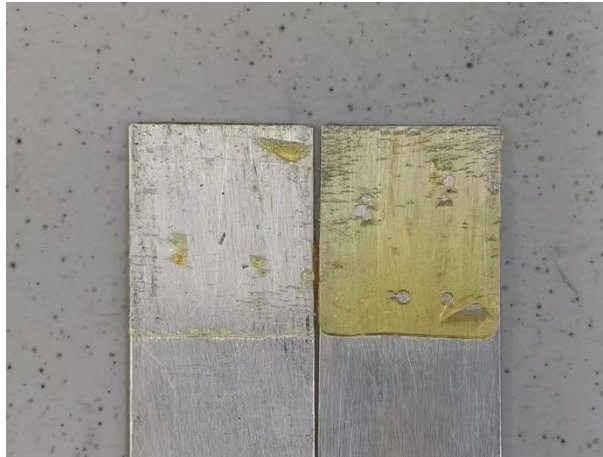
Figure S4. The failure mode of the adhesive lap joint of PTAE.
