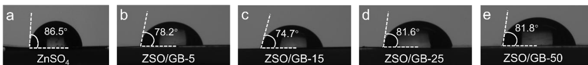
Figure S5. Contact angles of (a) the \text{ZnSO}_4 , (b) the ZSO/GB-5, (c) ZSO/GB-15, (d) ZSO/GB-25 and (e) ZSO/GB-50 electrolytes. Compared to the \text{ZnSO}_4 electrolyte, \text{ZnSO}_4/\text{GB} hybrid electrolytes exhibit smaller contact angles on the zinc foil, demonstrating a favorable zinc affinity. Note that the \text{ZnSO}_4/\text{GB} hybrid electrolytes with high GB concentrations, such as 50 mM, show relatively large contact angles. This is because the \text{ZnSO}_4/\text{GB} hybrid electrolytes with high GB concentrations possess relatively high viscosity to reduce their fluidity, thereby showing an increased contact angle on zinc anodes.
