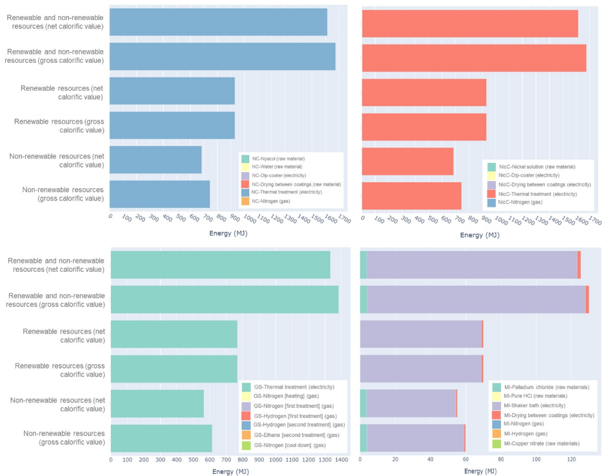
Figure SI 15 - Primary energy demand results for each stage related to CVD_Pd_200_Cu synthesis (NC, NicC, GS and MI).
