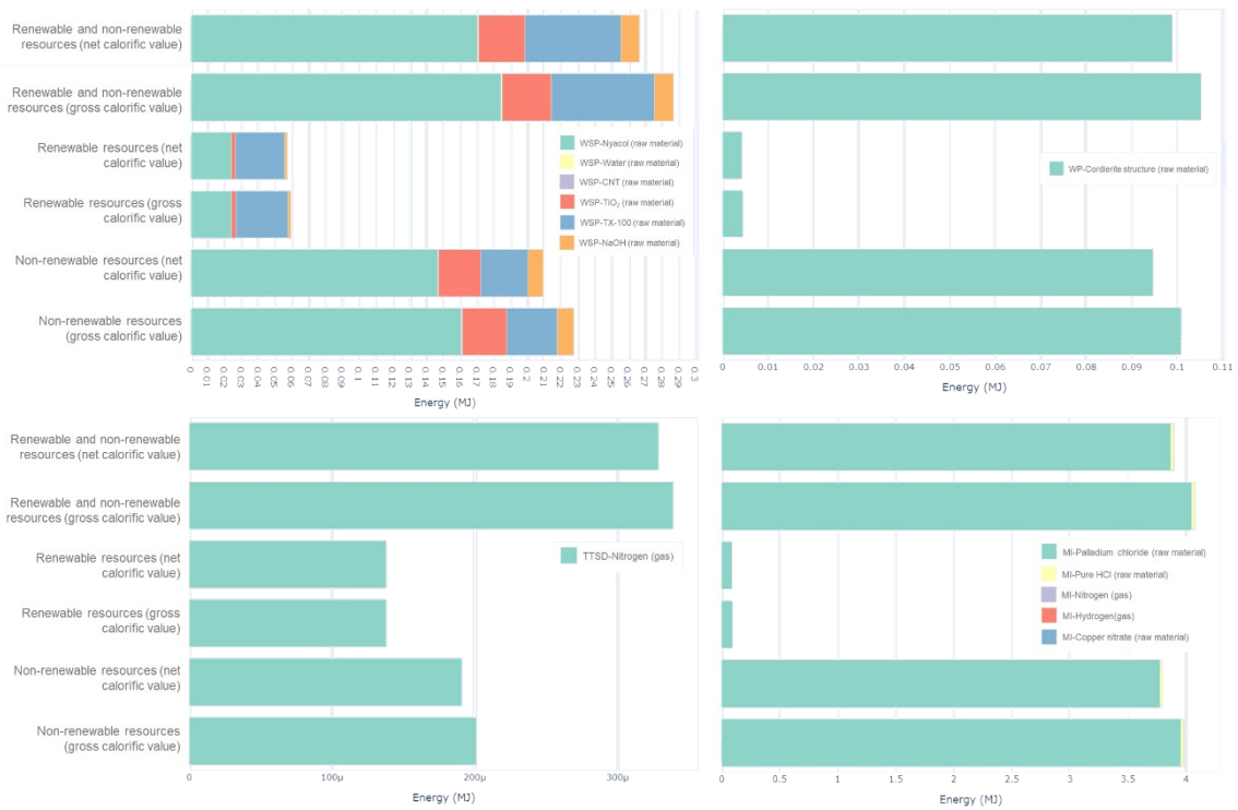
Figure SI 9 - Primary energy demand impacts of WCP(CNT:TiO 2 ) 550 Pd 200 Cu synthesis for each stage WSP, WP, TTSD and MI) excluding inputs related to energy consumption.
