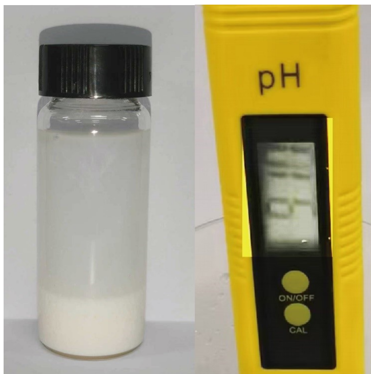
Fig. S4. Photos of directional precipitation of \text{Pb}^{2+} into \text{Pb}(\text{OH})_2 by pH control.
