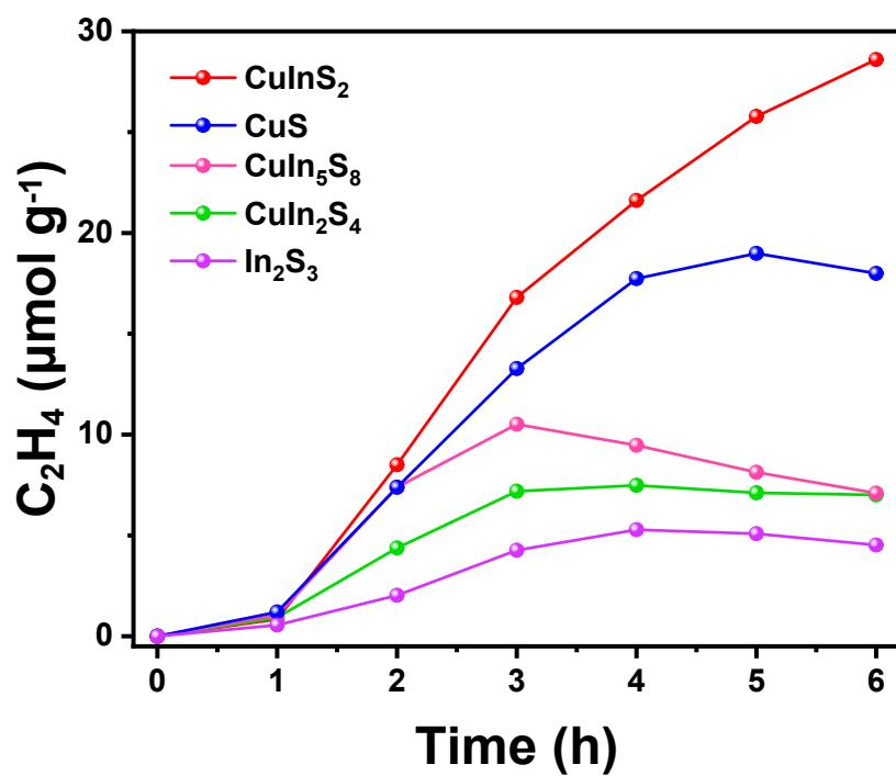
**Fig. S4** Evolution of  $\text{C}_2\text{H}_4$  yield over time for different samples.
