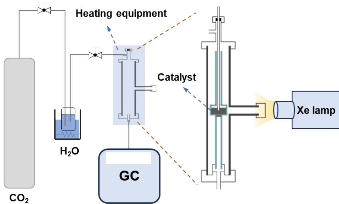
**Fig. S1** Flow chart of reaction device.
