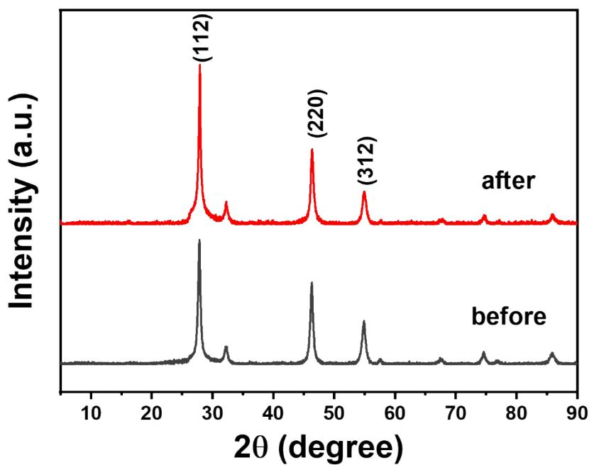
**Fig. S6** XRD pattern of  $\text{CuInS}_2$  sample before and after reaction.
