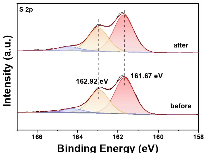
**Fig. S9** XPS spectra before and after reaction for CuInS<sub>2</sub> sample: S 2p.
