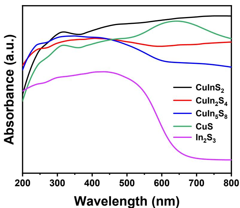
**Fig. S10** UV-Vis absorption spectra of the Cu<sub>x</sub>In<sub>y</sub>S.
