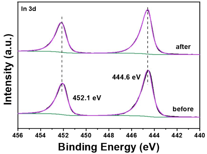
**Fig. S8** XPS spectra before and after reaction for CuInS<sub>2</sub> sample: In 3d.
