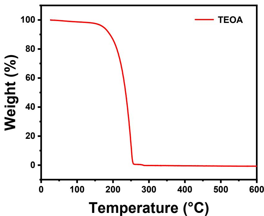
**Fig. S2** Thermogravimetry graph of TEOA in nitrogen atmosphere.
