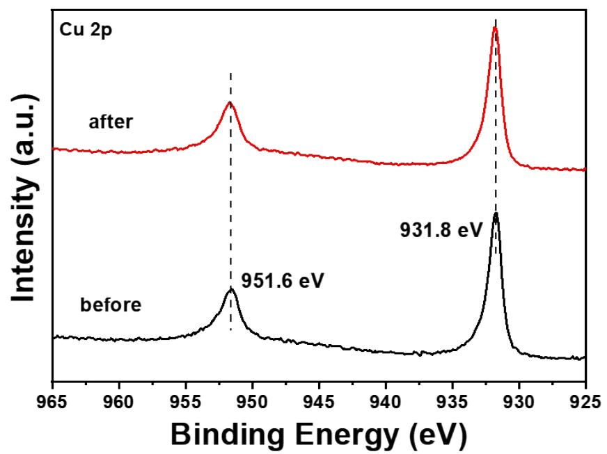
**Fig. S7** XPS spectra before and after reaction for CuInS<sub>2</sub> sample: Cu 2p.
