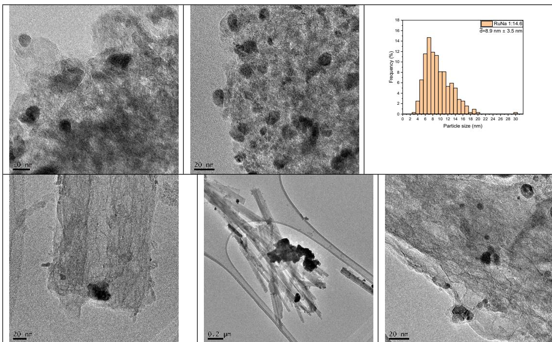
**Figure S3.** Representative TEM images and histograms for the DFMs with different Na loadings
