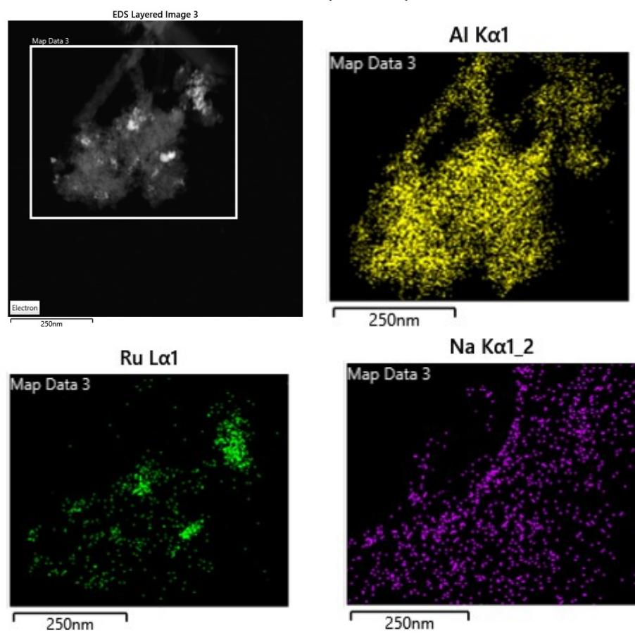
**Figure S4.** EDS mapping of the DFM with different Na loadings
