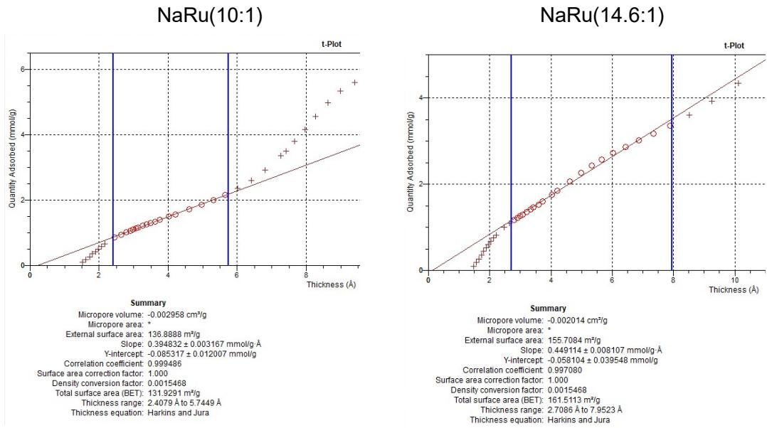
**Figure S2.** t-plot analysis of the N<sub>2</sub> adsorption isotherm for the different DFMs
