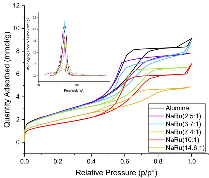
**Figure S1.** N<sub>2</sub> adsorption isotherms and pore size distribution (inset) for the different Na loadings
