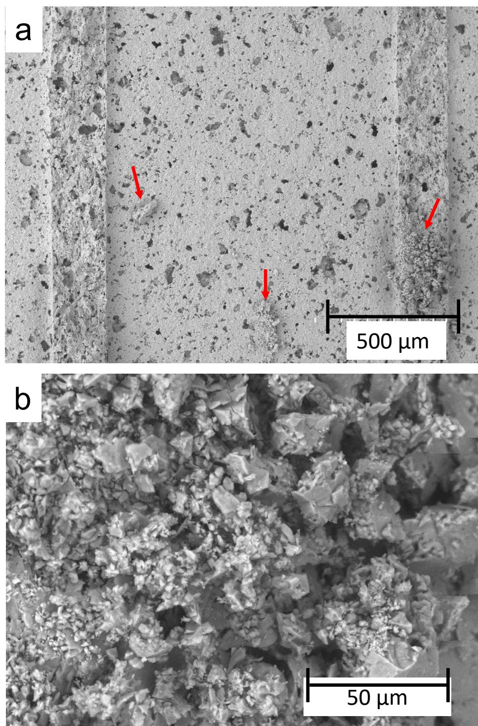
**Figure S5.** Representative SEM images of a longitudinal cut of a monolith channel coated with Alumina and after impregnation of DFM RuNa (8.3:1): (a) cut of a channel of the monolith; (b) magnification with a detail pointed out with red arrow in Figure S5a
