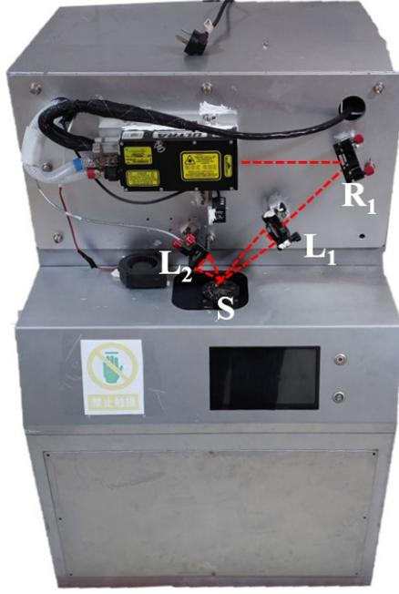
Fig.S1. The off-line LIBS machine, R1: mirror, L1/L2: lens, S: sample stage
