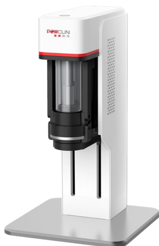
Fig. S1 The pressure-driven sample loader. This loader precisely regulates solution flow rate through air pressure and uses PEEK tubing to minimize metal ion contamination. It also reduces settlement and aggregation of particulate samples by agitating and rotating the sample tubes.
