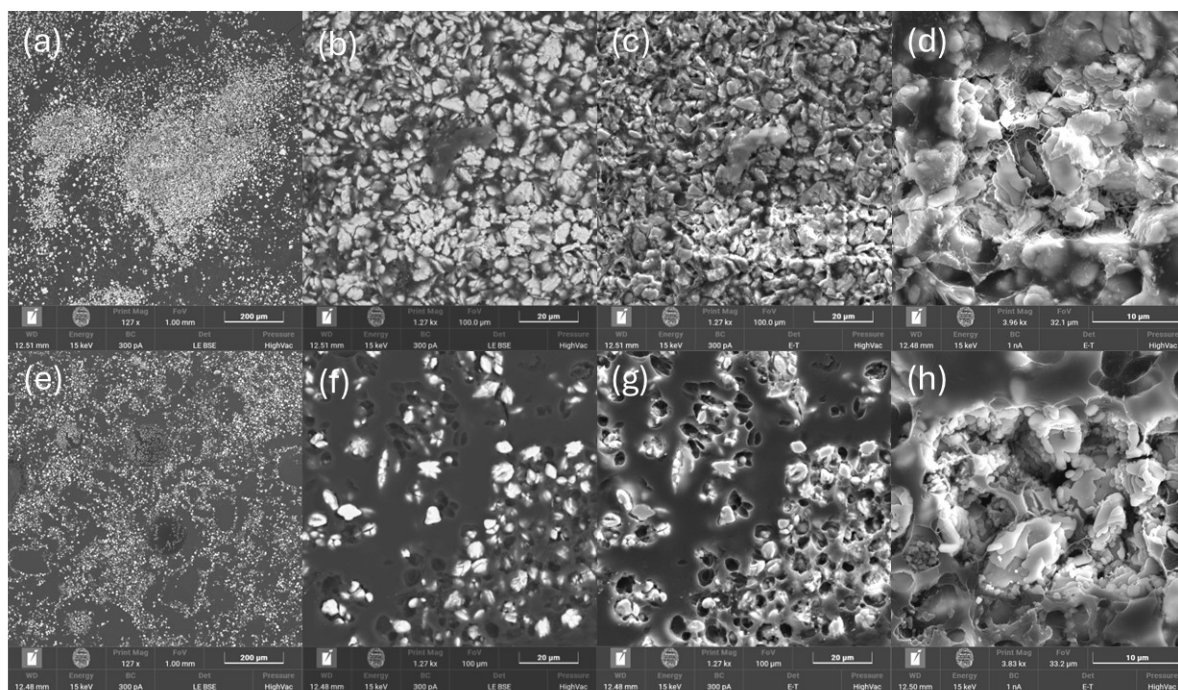
Figure SI-2: SEM (a), (c) et (d) SE and (b) BSE images of reference material A with 2.89 \mu\text{g.g}^{-1} of ^{226}\text{Ra} and SEM (e), (g) and (h) SE and (f) BSE images of reference material B with 9.65 \mu\text{g.g}^{-1} of ^{226}\text{Ra} , with table results of O, S, Cl and Ba (at%) beside obtain from some area analyzed of the blank and reference material A and B. SE images (d) and (h) show area analyzed by NanoSIMS.
