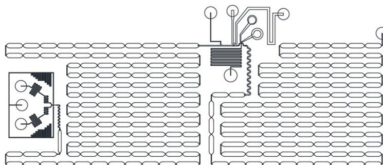
**Figure S4:** Initial microfluidic chip design, encompassing droplet co-encapsulation, an initial 10-minute droplet incubation, picoinjection and a subsequent 8-minute droplet incubation.
