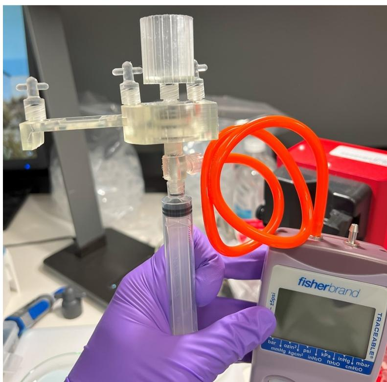
Figure S5. Setup for vacuum measurements.
