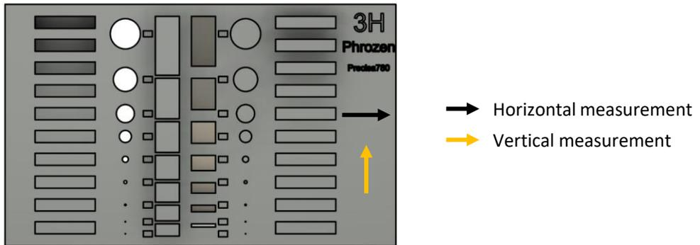
**Figure S14.** Visual representation of average roughness measurements. Three vertical and three horizontal measurements were performed and averaged on each 3D printed characterisation platform to recapitulate its overall average surface roughness.
