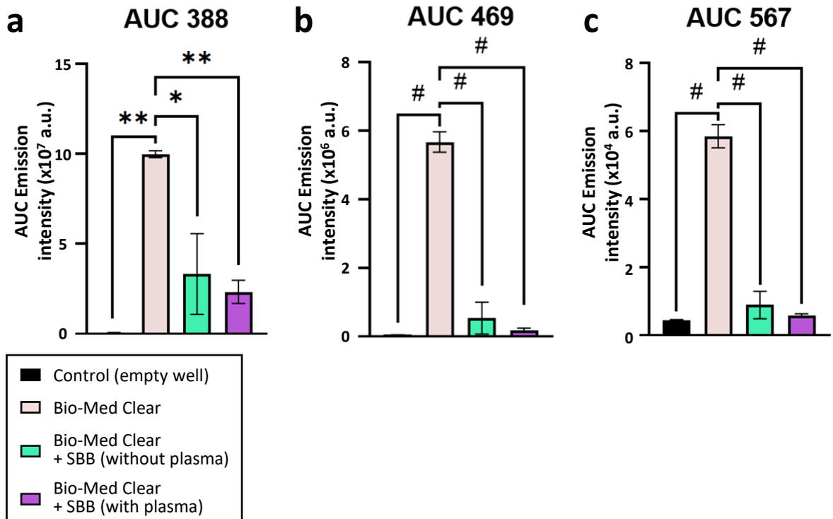
**Figure S4.** Area Under the Curve (AUC) measurements based on Excitation – Emission spectra of untreated and treated 3D-printed Bio-Med Clear. 3D-printed inserts of untreated or SBB and SBB + plasma O<sub>2</sub> treated Bio-Med Clear were excited at **(a)** 388 nm, **(b)** 469 nm and **(c)** 567 nm.
