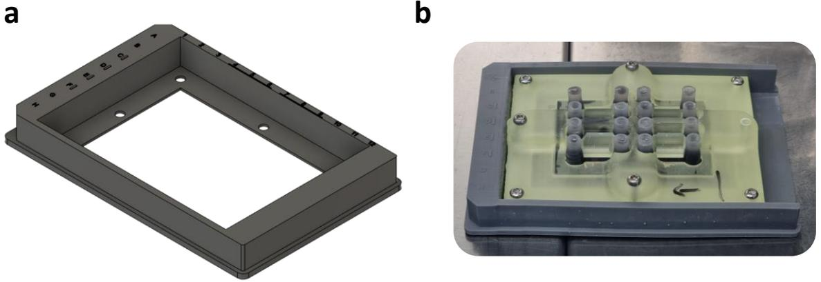
**Figure S5.** Custom plate adaptor for positioning the microfluidic chip in 96-well format for robotic use or automated microscopy. (a) Design of the plate adaptor and (b) microfluidic chip inserted in the plate adaptor.
