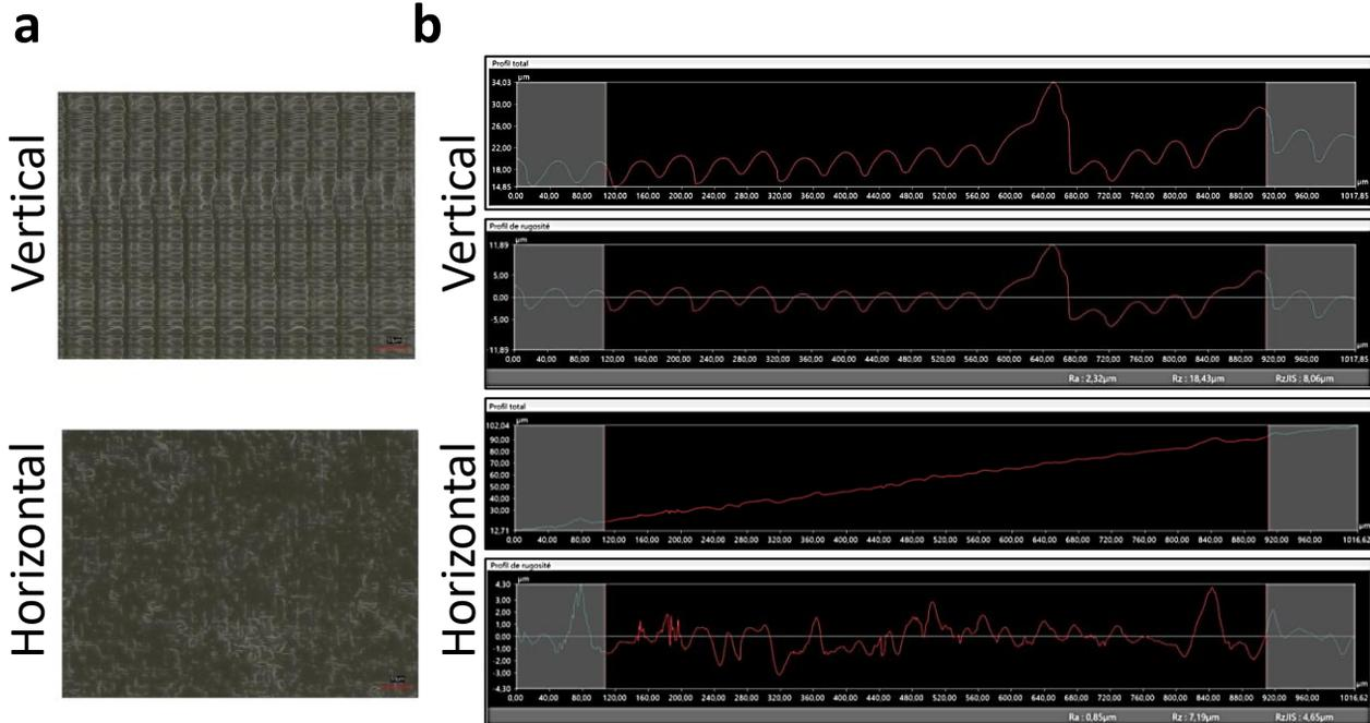
**Figure S2.** Surface roughness imaging and profiling using digital microscopy depending on printing orientation, showing the printing resins layers (example of AquaClear printed with LCD printer). **(a)** Images at 500X magnification. **(b)** Surface height profile, raw and corrected.
