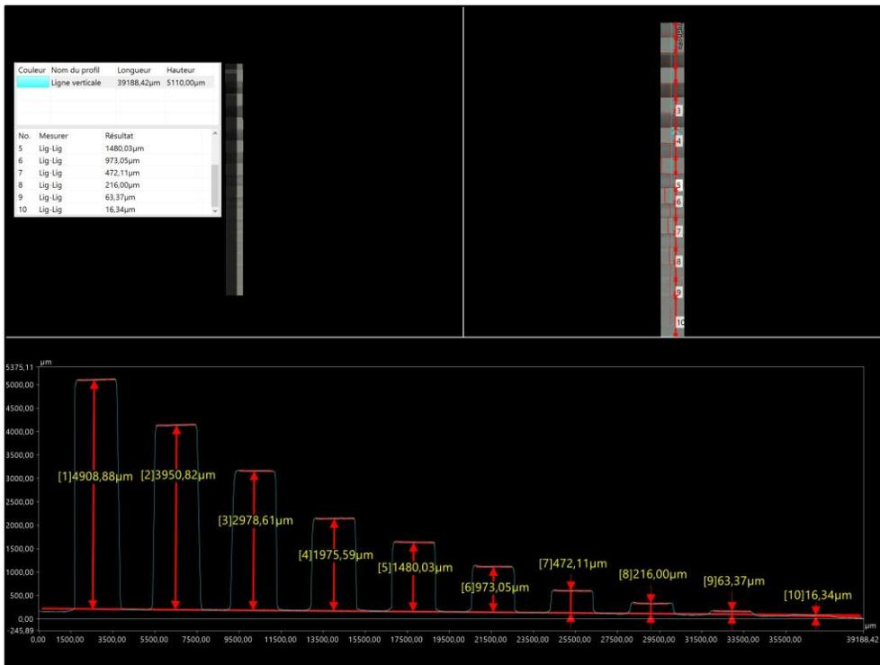
**Figure S11.** Example of a height profile measurement with the digital microscope on protrusions.
