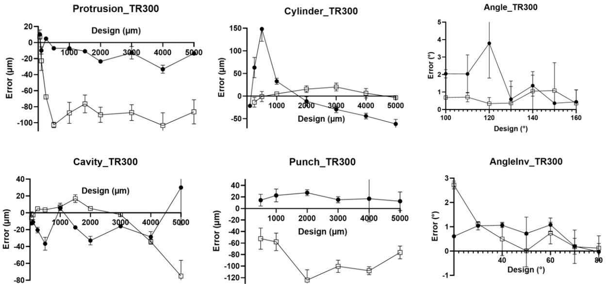
**Figure S12.** Example of all the measurements obtained for the different patterns to characterise the precision of a resin, depending on printing orientation. Data are presented as mean values +/- standard deviations (n=3).
