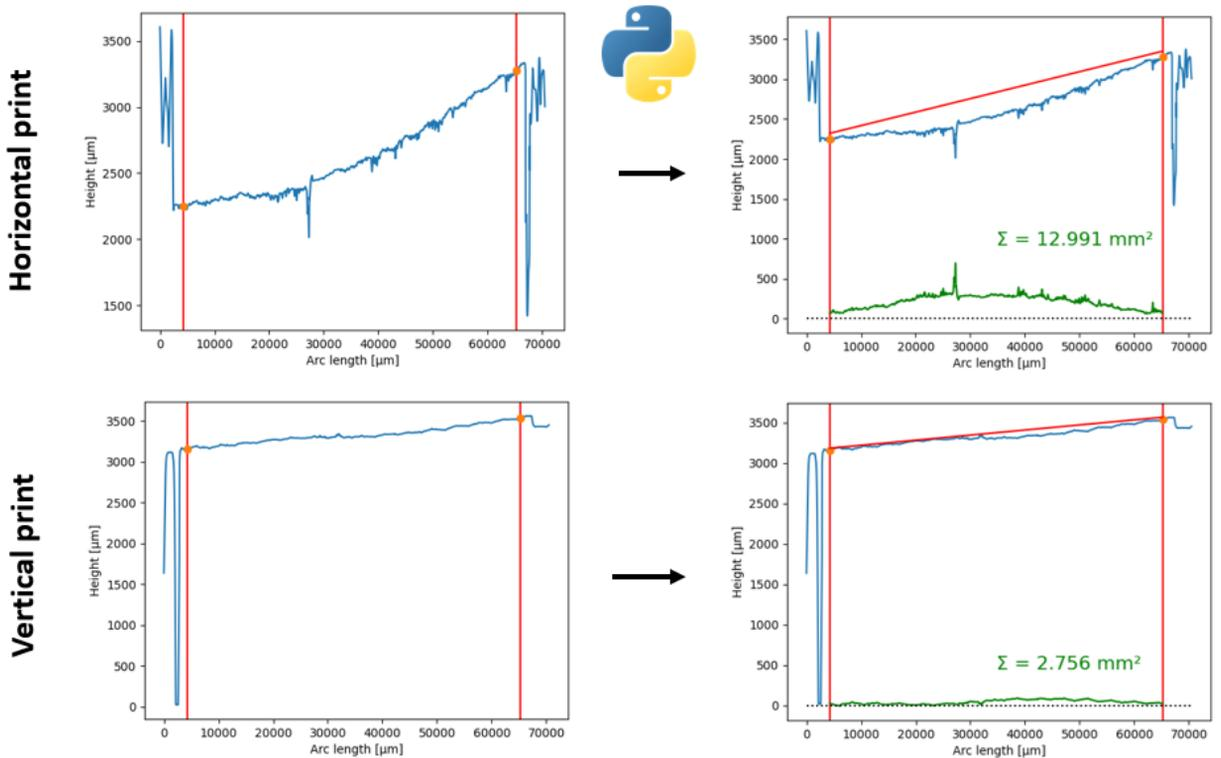
**Figure S13.** Methodology for curvature characterization, determination of area using height profile extracted from digital microscope measurement and automated analysis thanks to a custom python script.
