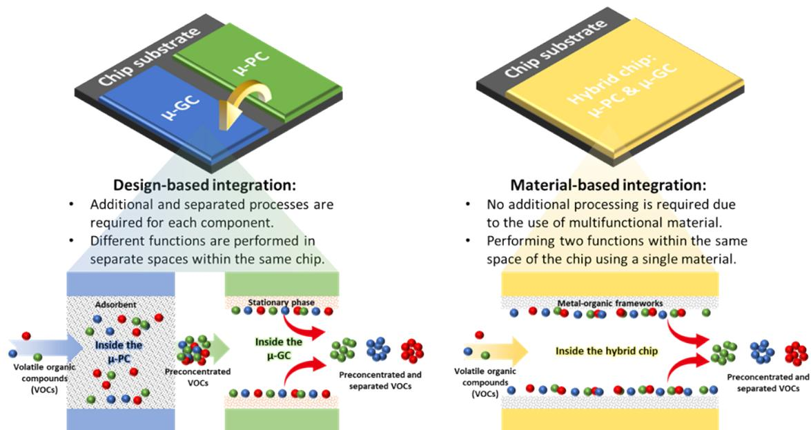
**Fig. S1** Schematic illustration highlighting the difference between design-based integration and material-based integration.
