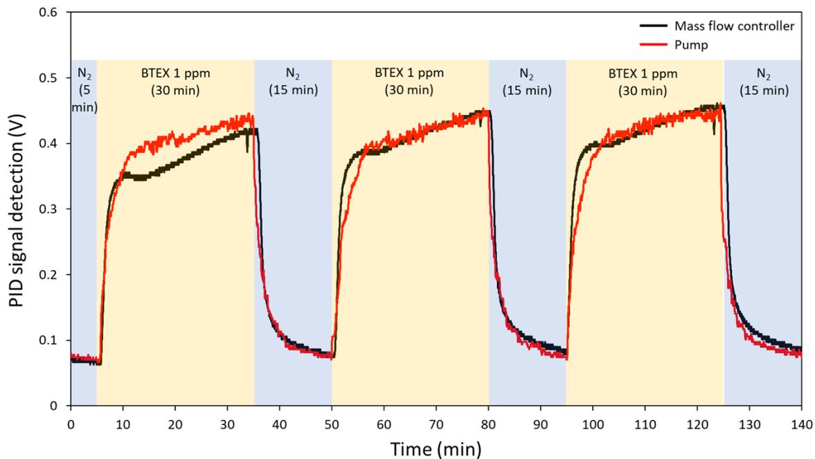
**Fig. S4** Results of the pump contamination test. When using the mass flow controller (MFC), the flow direction was MFC → uncoated hybrid chip → PID (4 mL·min<sup>-1</sup>). When using the pump, the flow direction was Tedlar bags → three-way valve → pump → uncoated hybrid chip → PID (4.08 mL·min<sup>-1</sup>).
