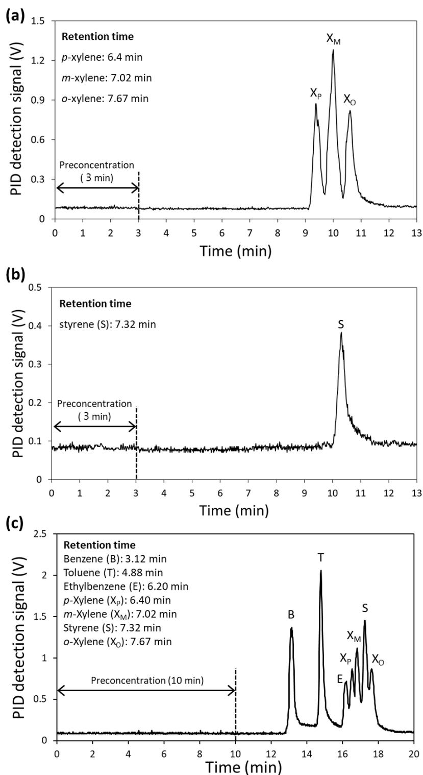
**Fig. S8** Experimental results for xylene isomers, styrene and monocyclic aromatic hydrocarbons obtained using the hybrid GC platform. (a) Chromatogram of xylene isomers from a gas cylinder containing a mixture of xylene isomers, (b) chromatogram of styrene from a single gas cylinder, and (c) chromatogram of monocyclic aromatic hydrocarbons.
