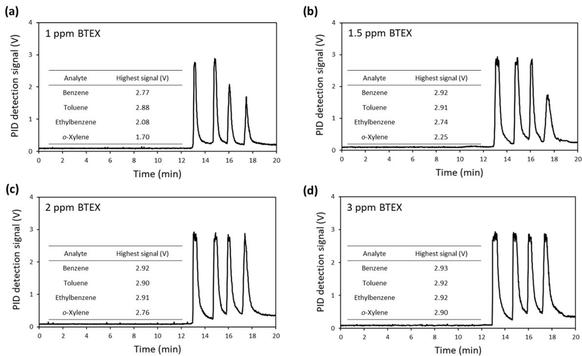
**Fig. S6** Experimental results for various concentrations of BTEX to determine the linear range. (a–d) Chromatograms of 1, 1.5, 2, and 3 ppm BTEX, respectively, including the highest PID detection signal for each analyte peak.
