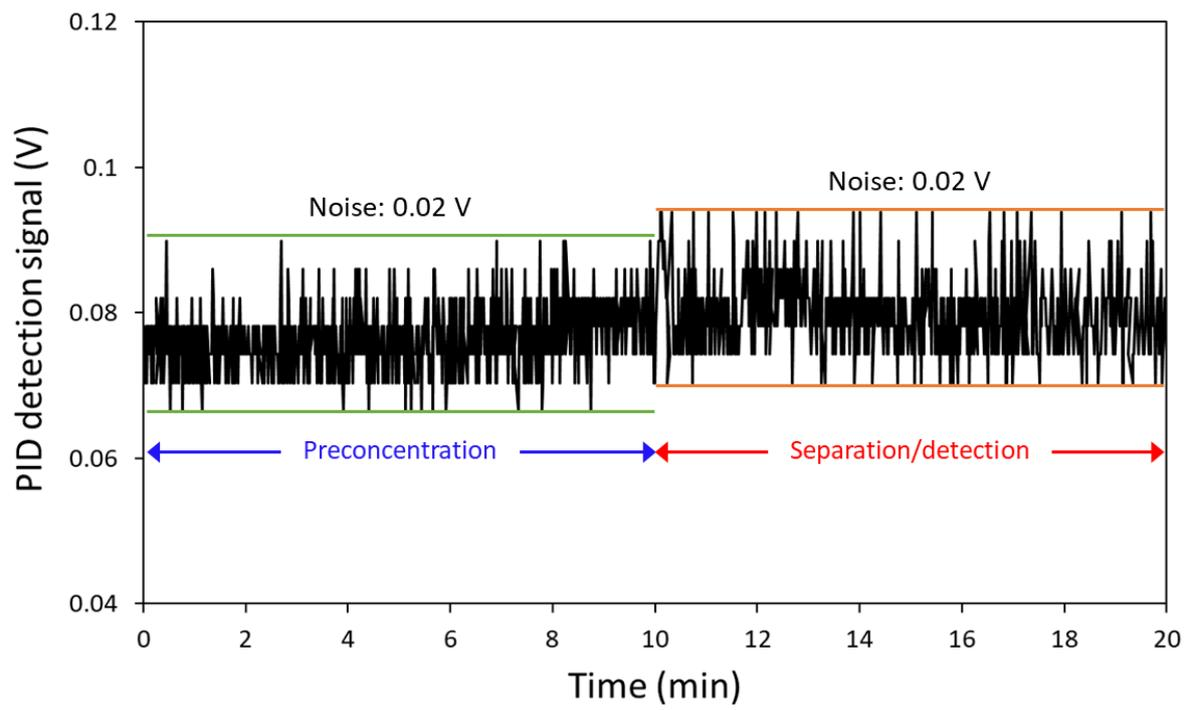
Fig. S7 Noise levels measured in the blank test.
