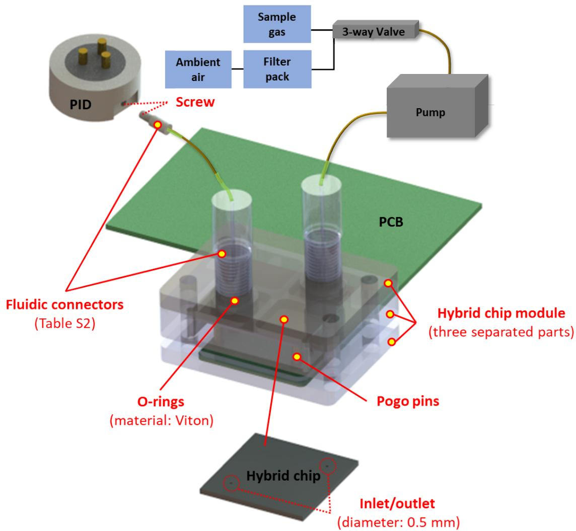
**Fig. S2** Detailed interconnections between components in the hybrid GC platform.
