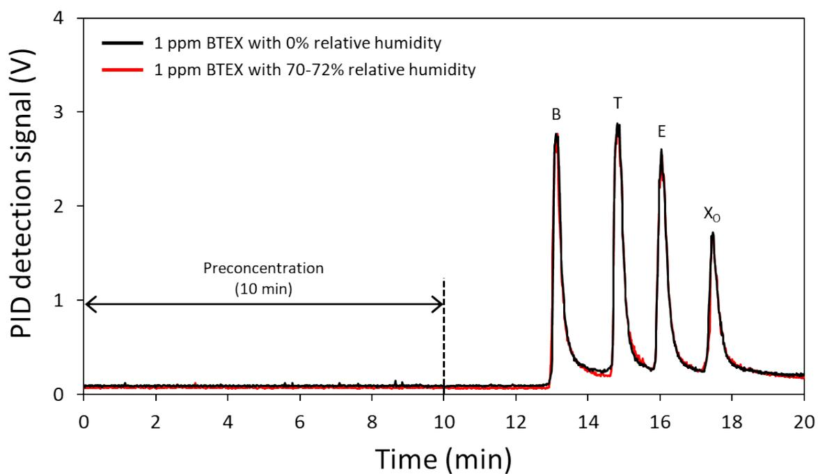
**Fig. S11** Effect of relative humidity on analytical performance. The relative humidity level of 70–72% was achieved by placing a water bubbling chamber (a conical tube) between the pump and the hybrid chip.
