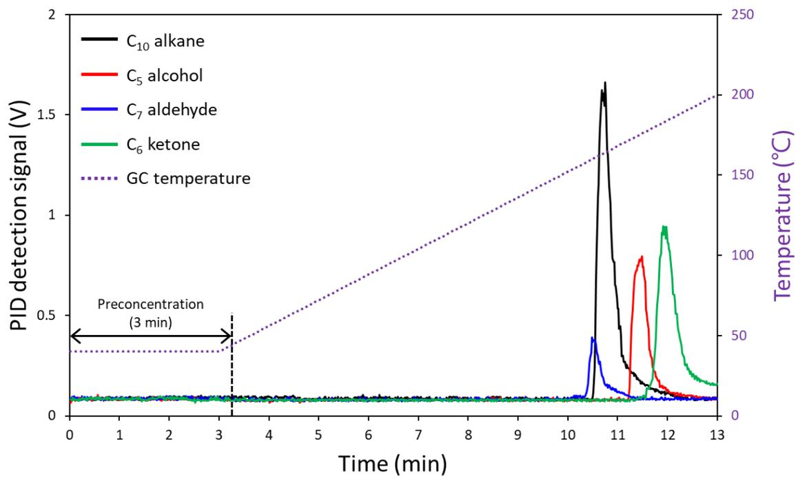
**Fig. S10** Desorption and detection of analytes undetected in Fig. 6 due to insufficient TD temperature (hybrid chip temperature ramping: 40°C to 200°C).
