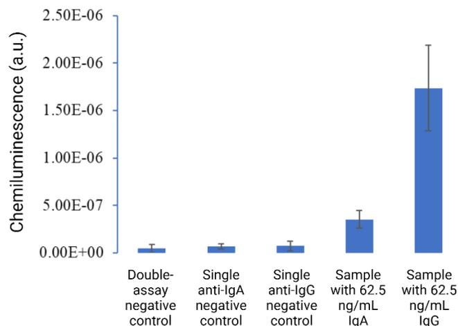
**Figure S8.** Bar plot of the chemiluminescent signal generated from digital microfluidic assays for the double-assay negative control (for host IgG and IgA in saliva), the conventional single-assay control for host IgA in saliva, the conventional single-assay control for host IgG in saliva, saliva spiked with 62.5 ng/mL host IgA, and saliva spiked with 62.5 ng/mL host IgG. Error bars represent  $\pm$  one standard deviation for  $n=3$  replicates per condition.
