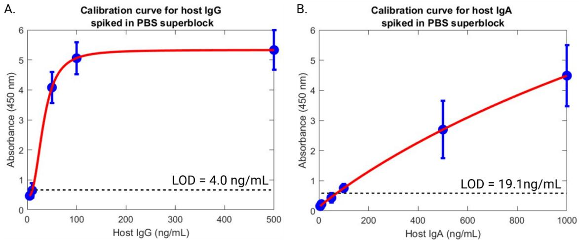
**Figure S6.** Plots of off-chip immunity assay measurements (blue markers) as a function of (A) host IgG and (B) host IgA spiked in PBS SuperBlock™. The curves are 4PL fits to the data, and the dashed lines illustrate the LODs of 4.0 ng/mL (IgG) and 19.1 ng/mL (IgA), respectively. Error bars represent  $\pm$  one standard deviation for  $n=3$  replicates per condition.
