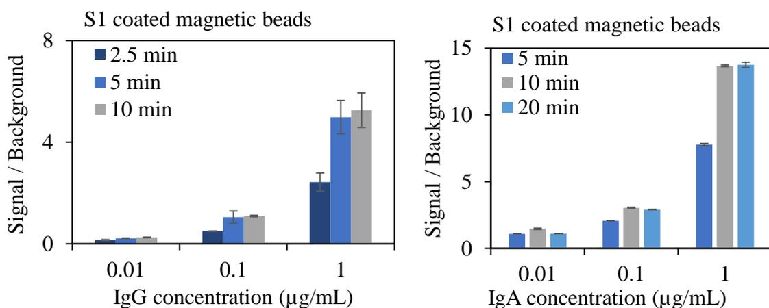
**Figure S5.** Optimization of sample incubation time for off-chip immunity assays. Bar plots of signal-to-background ratio as a function of host IgG concentration (left) and IgA concentration (right) spiked in PBS SuperBlock™ after incubation for 2.5 (dk. blue), 5 (med. blue), 10 (grey), or 20 (lt. blue) min. Error bars represent  $\pm$  one standard deviation for  $n=3$  replicates per condition.
