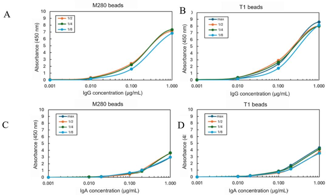
**Figure S4.** Off-Chip optimization of bead size and bead coating capacity for off-chip immunity assays. Semilog plots of assay signal as a function of host IgG (A, B) and host IgA (C, D) concentration, spiked in PBS SuperBlock™ for M280 (A, C) and T1 (B, D) beads modified with S1 at 1/8 (light blue), 1/4 (green), 1/2 (orange), and ‘maximum’ (dark blue) binding capacity.
