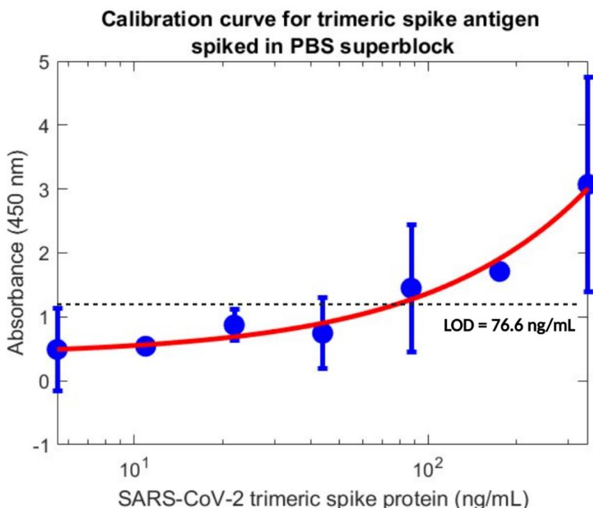
**Figure S3.** Semilog plot of off-chip infection assay measurements (blue markers) as a function of SARS-CoV-2 trimeric spike protein concentration spiked in PBS SuperBlock™. The curve is a 4PL fit to the data, and the dashed black line illustrates the LOD of 76.6 ng/mL. Error bars represent  $\pm$  one standard deviation for  $n = 3$  replicates per condition.
