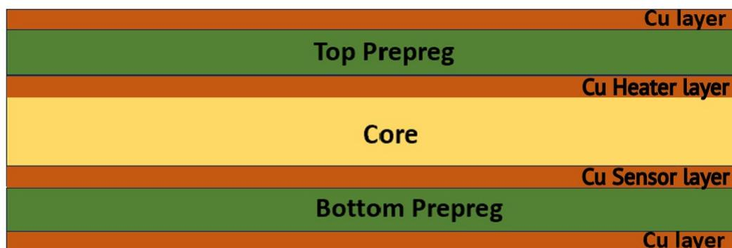
Figure S2: Four-layer PCB configuration used for manufacturing the PCB EWOD chip. Two inner copper layers are used for the heater–sensor pair.
