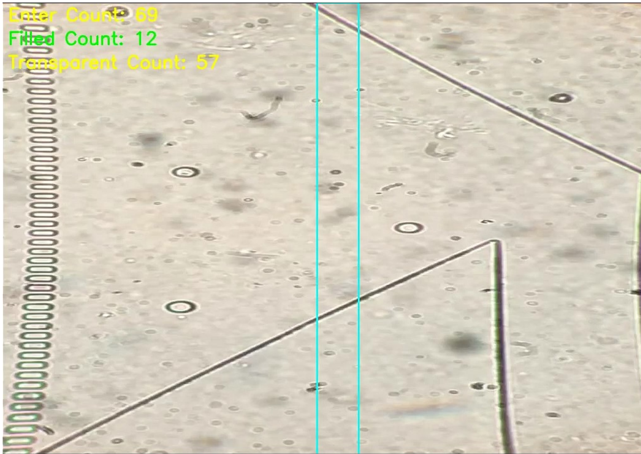
Movie S1. Cell counting using magnetic-activated smartphone microflow cytometry. The video was recorded at 239.98 fps and is displayed at 30 fps, resulting in slow-motion visualization of cell movement.
