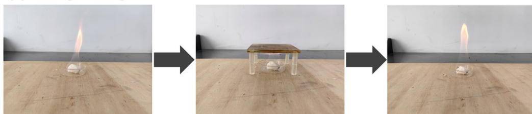
Fig. S13. Fire suppression performance of the microcapsule-based patch at different extinguishing distances: (a) 1 cm. (b) 2 cm. (c) 3 cm.
